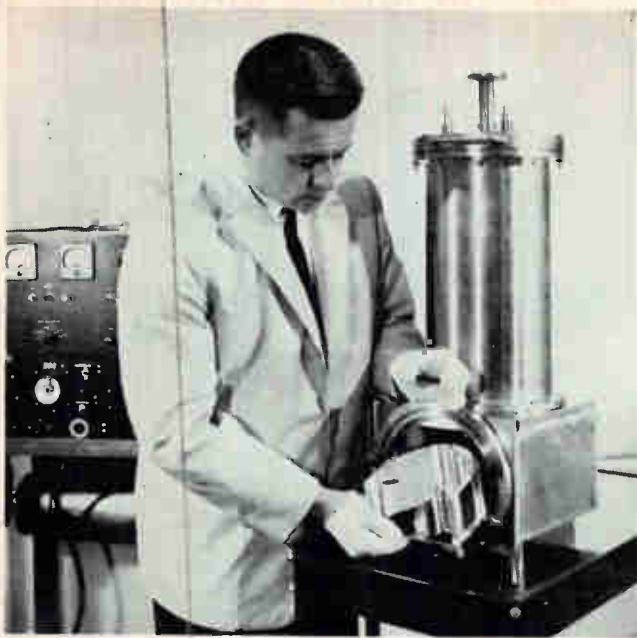
FIG. 9—Adjusting a cryostat laser. This laboratory device tests laser materials and excitation sources. Drawing shows details of the device (Raytheon)
