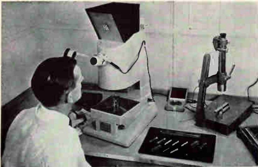
Interference fringes on the optical-interferometer screen check the end faces of a ruby rod for flatness within 1/20 of a sodium wavelength. Instrument at right checks parallelism of end faces to within 1 second of arc. On table are ruby rods and three rough cuts from ruby disc boules
