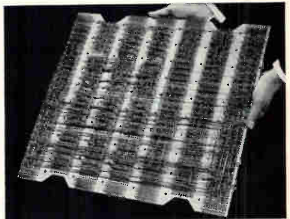
Complicated back panel—automatically wired by "Wire-Wrap" machine contains 2480 wires and 4960 connections.
