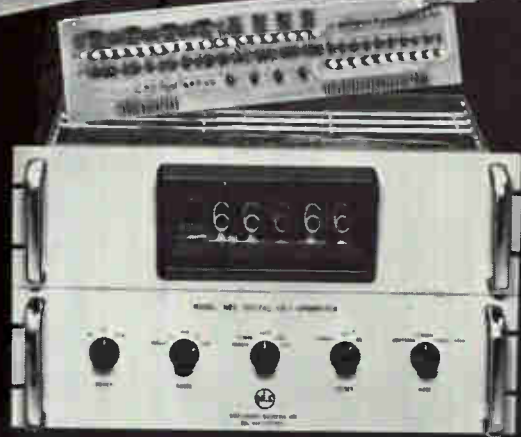
Digital voltmeters — originated by NLS — permit rapid and accurate voltage measurements. New Series 20 unit — with one plug-in decade board removed — shows the use of Allen-Bradley fixed resistors.
