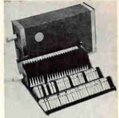
Component-carrying chips wrap around heat exchanger
