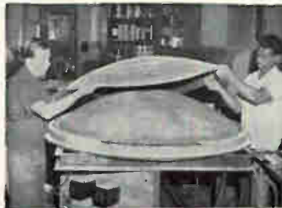
Preformed honeycomb is placed on the plastic covered foil, providing the structure with strength and rigidity
