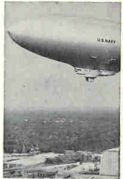
Flying wind tunnel allows Navy to test aircraft suspended below airship's cab.
