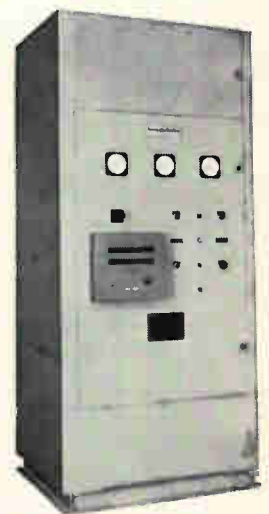
ABOVE — STATIC POWER RECTIFIER Output: 500 KW, 500 volts DC 1000 amperes Input: 13,800 volts, 33 amp. 3 phase, 60 cycle
