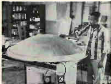
Foil reflector surface, 0.002 inch thick, is made ready
