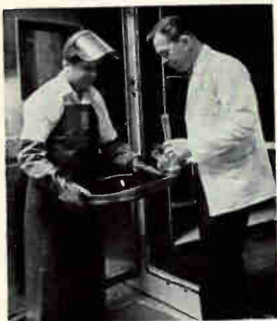
Motorola shaves know-how on putting 23-inch color inside black and white tube. Faceplate preparation (left) includes washing in hydrofluoric acid solution, preparing panels for phosphor coating (center), and fitting shadow mask in position (right)
