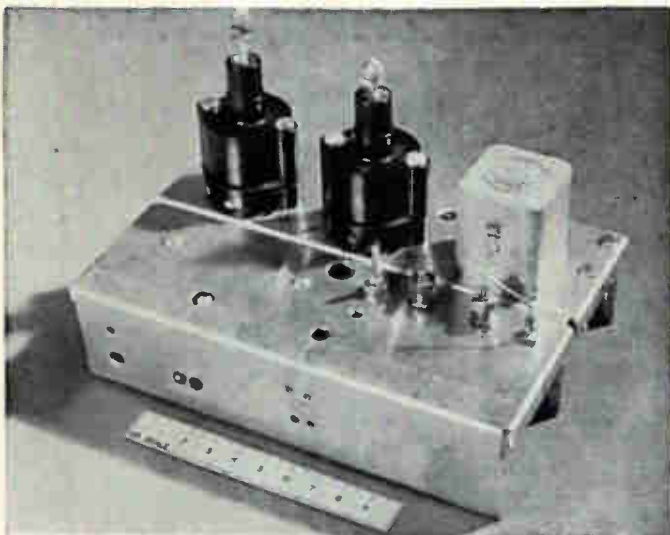
Chassis in photos above is small enough to fit inside clock case, which additionally contains miniature batteries and clock motor. Frequency controlling crystal is vacuum enclosed for minimum value (500 ohms) of series resistance
