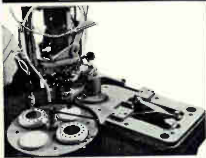
FOIL-DICE BONDER — Equipped with new automatic foil feed and indexing heat columns, machine positions and bonds both foil and dice on semiconductor headers. K&S Model 604 (not shown) available without foil feed.
