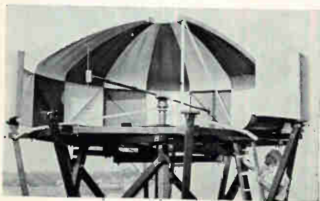
Rotating antenna of automatic direction finder is seen in partially assembled glass fiber radome
