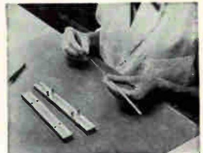
Mandrel is withdrawn after helix is attached to support rods
