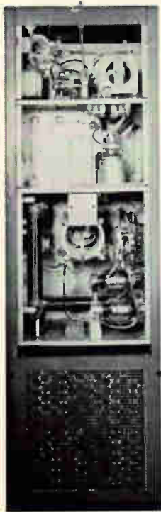
Gates Radio Company Broadcast Transmitter utilizing Jennings type M-100 and M-750 Vacuum Fixed Capacitors.
