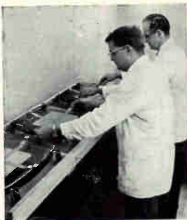
Motorola shaves know-how on putting 23-inch color inside black and white tube. Faceplate preparation (left) includes washing in hydrofluoric acid solution, preparing panels for phosphor coating (center), and fitting shadow mask in position (right)
