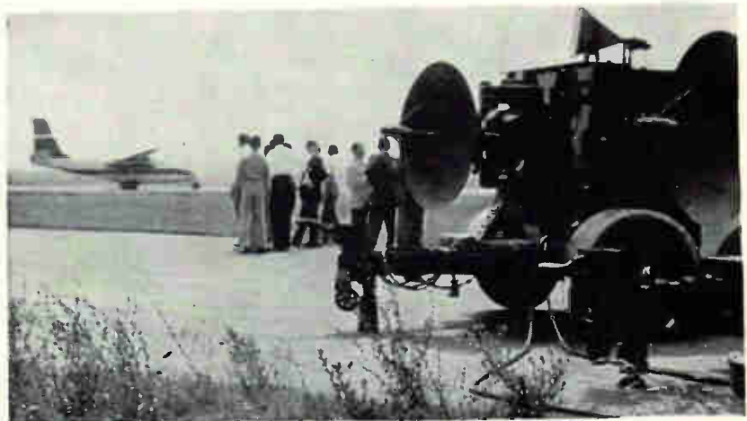
Bell Aerosystems Company reports successful flight tests of an automatic landing system developed for the Air Force. Coded commands in the radar beam serve as the data link and an S-band beacon is used for automatic tracking. Ground equipment includes tracking radar (above)
