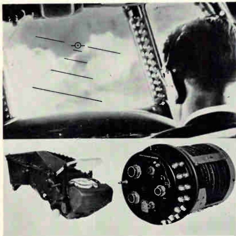
Optical projection of cathode ray display by new system (below) lets pilot see his attitude without looking down at instrument panel
