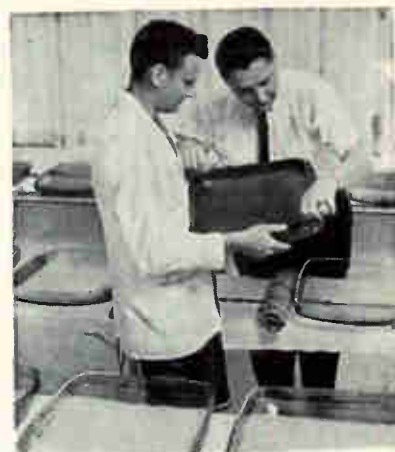
Motorola shaves know-how on putting 23-inch color inside black and white tube. Faceplate preparation (left) includes washing in hydrofluoric acid solution, preparing panels for phosphor coating (center), and fitting shadow mask in position (right)
