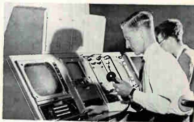
Radar display combines radar picture with identifying symbols, range rings, video map and azimuth marks
