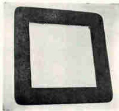
FIG. 2—The 6 inch by 6 inch electroluminescent converter panel and viewing screen
