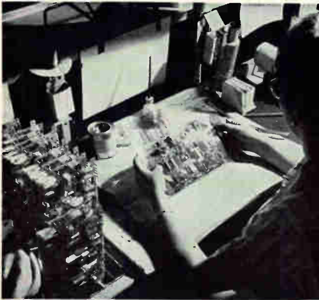
Plastic overlay is used by assembler (left) to check progress. Components to be added at each step are outlined in full size on the template; component polarity markings are indicated; wires, etc., are shown in color. Typical plastic overlay (right) for installing five diodes, and a drawing of the complete circuit
