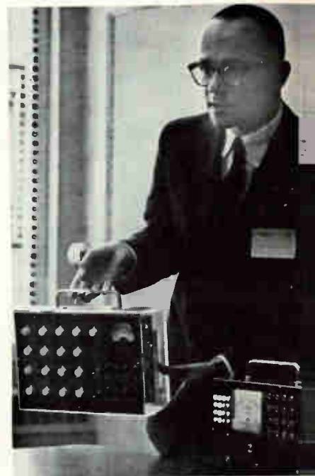
Bernard Widrow shows a conceptual version of Adaline called "Knobby Adaline". It uses rheostats instead of memistors. Plus or minus voltage settings of the knobs are quantized on the meter
