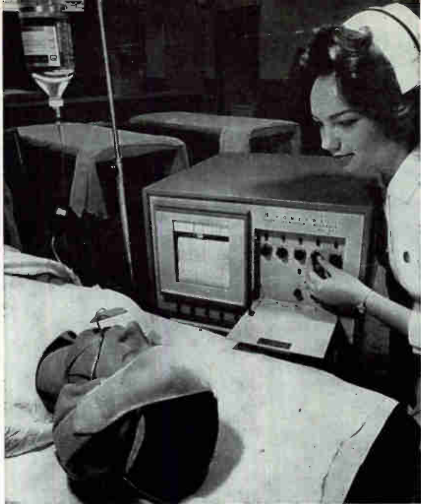
Nurse adjusts recorder-alarm controls of Minneapolis-Honeywell's body function monitor demonstrated at conference. Unit automatically measures and records temperature, pulse rate, respiration rate, and diastolic and systolic blood pressure of post-operative patient
