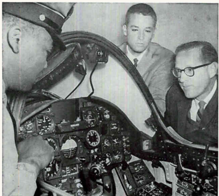
Link's aircraft simulator for Navy F8U-2N Crusader drills pilot in instrument flight, normal and emergency action. Instructor can monitor all pilot responses
