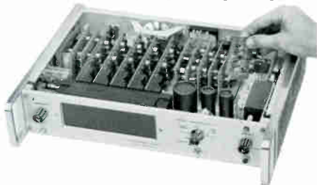
Note clean, compact, easy-to-service physical arrangement of new \Phi solid-state counters.
