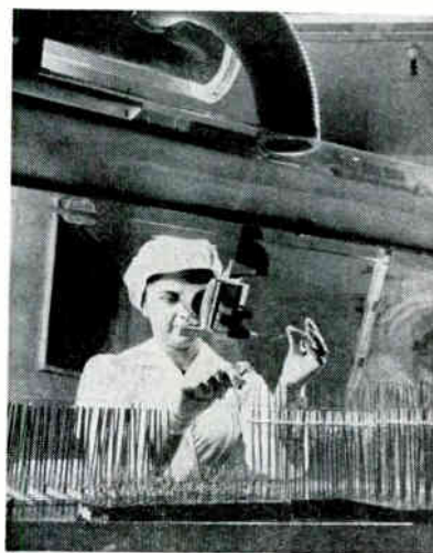
Coaxial pencil-type vacuum tubes by RCA are assembled with aid of microscope. Two were used in American astronaut's spacecraft for communication purposes
