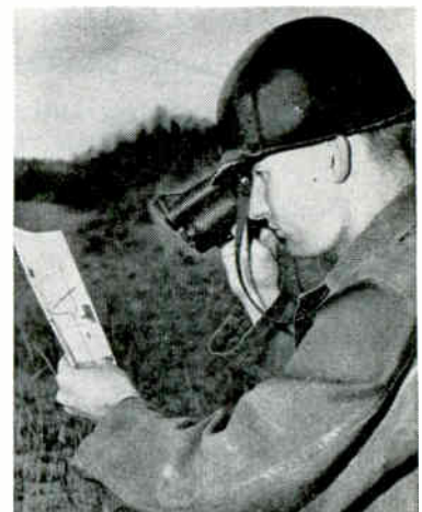
Transistorized infrared viewing device for military use was made by Varo Inc.
