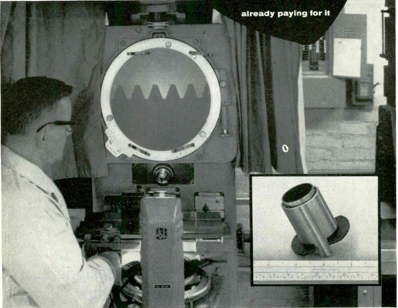
Unretouched photo (above) shows this cylindrical rack being inspected at 62.25X. Photo, courtesy of Baird-Atomic Inc., Cambridge, Mass.
