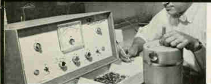
The Scintiscaler is a super-sensitive Geiger counter which monitors Radiflo leak test units
