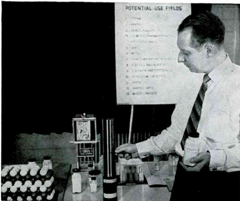
John Bugosh, of Du Pont, found that basic aluminum ions in solution can be polymerized in a controlled manner to produce colloidal particles which are not much larger than organic polymer molecules. Significance: thermal, insulating, conducting, and optical properties that suggest interesting applications for metals, ceramics, laminates and electronic components
