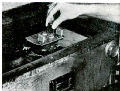
Assembly is placed on floating mask, with board and mask edges mating
