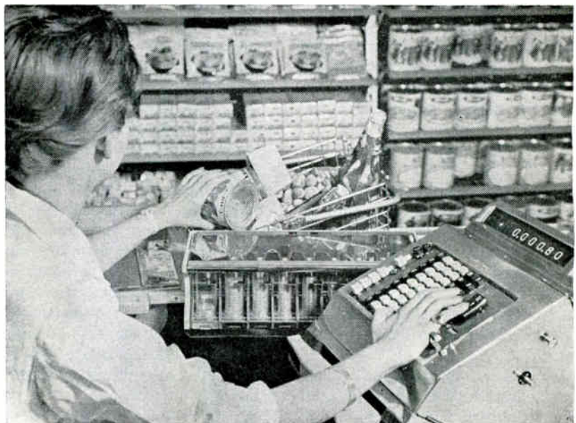
Input pulses from cash register activate Sweda's automatic coin changer and provide change to customer in this system developed in Switzerland
