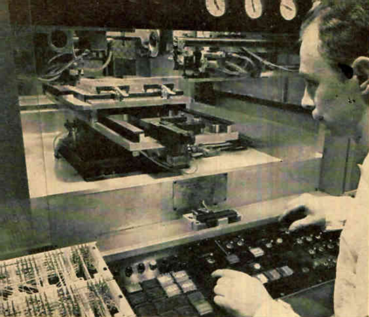
Automatic wire-wrap machine used at Honeywell's computer plant cuts, positions and connects a wire every six seconds. Device is punched-card controlled
