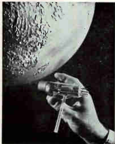
Ionization gage by Westinghouse has low mass elements that withstand space acceleration forces
