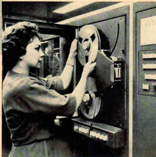
Videograph output unit built by A. B. Dick translates magnetic tape into edited output for an electrostatic label printer
