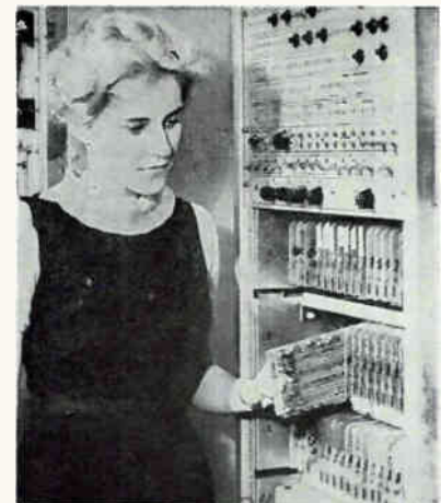
Data unit made by Siegler Corp. computes weather information for distribution by phone, radio
