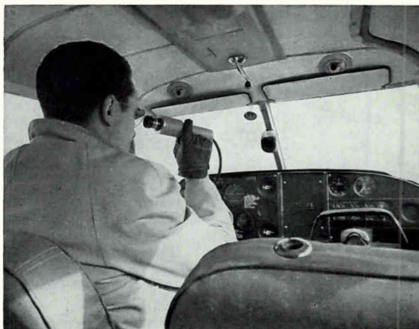
Miniature crt display device by Westinghouse allows telescope-type viewing of radar and tv data. It uses a 0.60-in tube, costs $150
