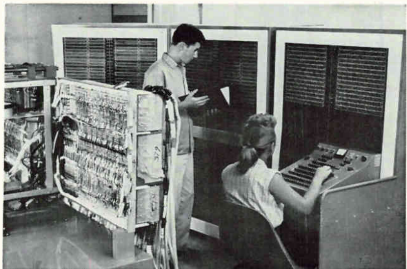
Wiring continuity tester recently introduced by Autonetics Division of North American Aviation, Downey, Calif., will test one to 20 wires per second, depending on number of wires to a connector pin. It uses a master, does not need programming. Consoles can be ganged
