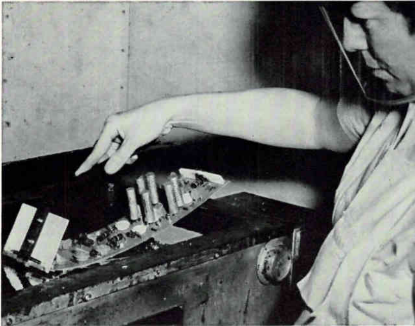
Rolling large boards keeps the solder surface hot and prevents tailing and bridging
