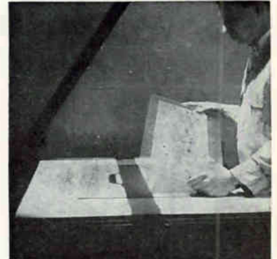
Contact printing the assembled template produces negative
