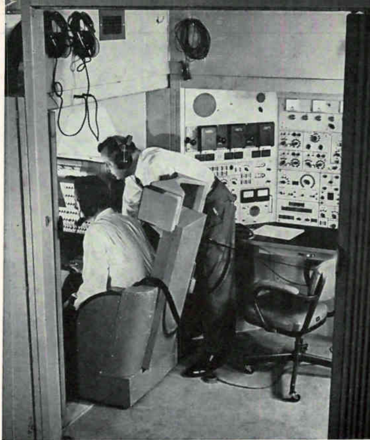
Instructor orients B-58 Defense System Operator in ecm simulator used at SAC bases
