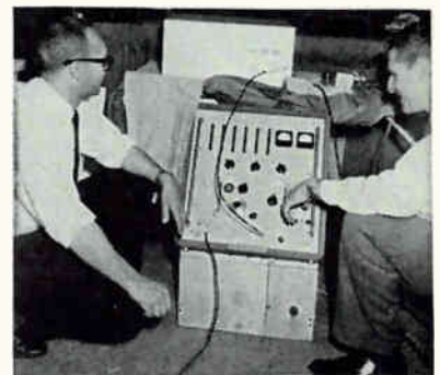
Rubidium frequency standard by STL has long-term stability of 1 part in 10 10 . Reference is optically pumped rubidium cell
