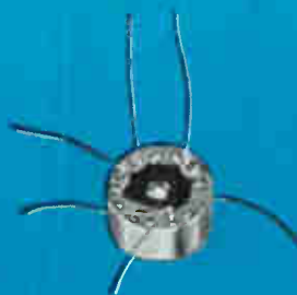
ACTUAL SIZE .228" high, .531 diam. COMPONENT DENSITY 324/in 3 (560,000/ft 3 )
