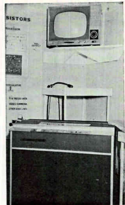
Video tape recorder by Sony is smaller than an office desk, uses 96 transistors. Tunnel diodes are used in memory head. Program showed a Japanese chorus line
