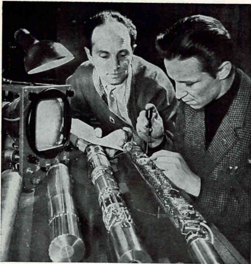
Soviet-designed television pickup unit for inspection of well sides uses semiconductors and miniature components. Metallic cylinder is 1,690 mm long, 60 mm in diameter (Sovfoto)
