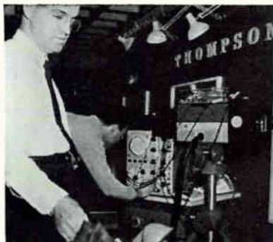
Image converter camera by STL converts optical image to electron beam, gates beam to achieve 2½-nanosecond exposure time
