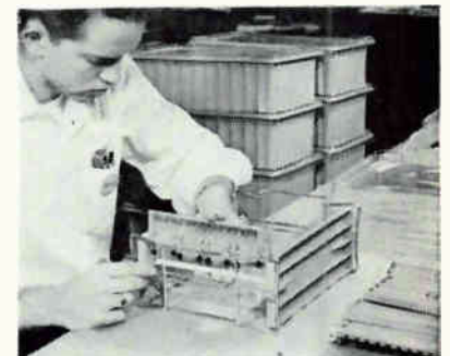
Board is fitted into wire and plastic insert of tote box
