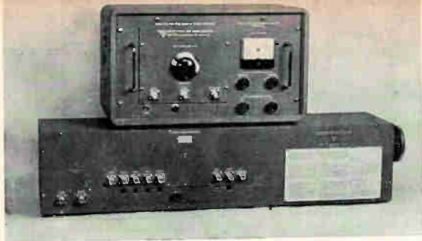
Phase detector for 15 Mc to 400 Mc. Upper cabinet contains balanced tuned amplifier, phase detector, and null indicator; lower cabinet contains coaxial variable delay line and four plug-in step delay lines for extending range of total delay
