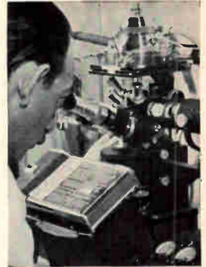
Creative engineering, applied to printed circuits, is exemplified by flush-circuit switching device (left), and a versatile resistor element (center). Steve Gulyas operates metallurgical microscope equipped with electric furnace (right), a significant tool in selecting proper materials for these circuits
