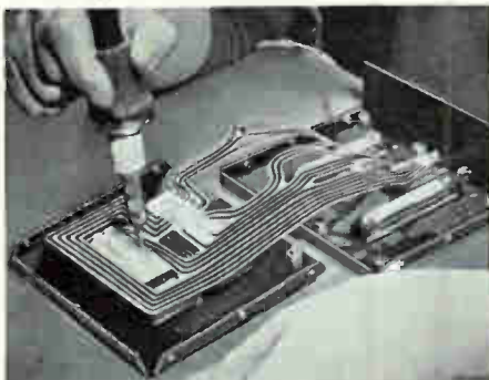
Assembly gets off to a fast start! One-piece Flexprint cables are self-positioning. They locate conductors and terminations with flawless accuracy. Each pierced termination pad automatically fits itself over its own connector pin. Wiring errors are almost impossible! And soldering becomes a high-speed operation because each connection is completely visible, not hidden in the connector or lost in a tangle of wires. Assemblers can see at a glance that each connection is tight and right.
