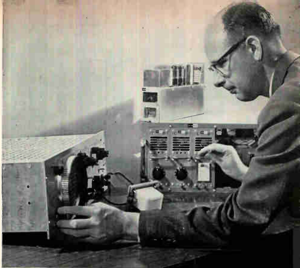
Author makes final adjustment on one of two wideband d-c amplifiers used to reject common-mode during differential amplification
