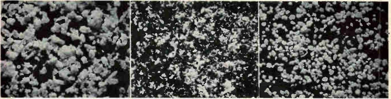
Photomicrographs, enlarged 5.5 times, illustrate the three powders used in the fabrication of TFE tape-wrapped and extruded wires. Particle sizes of TFE-1 (left); TFE-5 (center); and TFE-6 (right) are the key to the basic characteristics of the insulated wire
