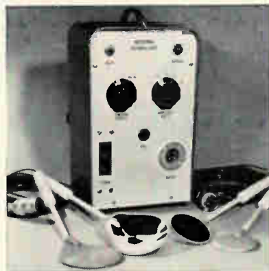
Portable defibrillator being marketed by Medtronic. Paddles in foreground have concave surfaces for maximum contact, insulated backs to limit application area and nylon handles to protect surgeon
