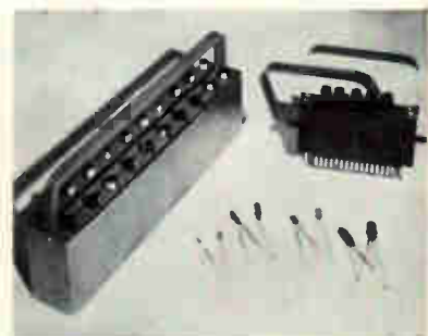
Magazine adapters. Newly-designed units at left hold 20 transistors
