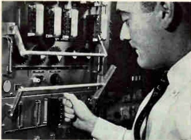
Interlock bar cuts off power before adapters can be inserted or removed
