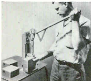
Welded handle extension gives punching leverage
