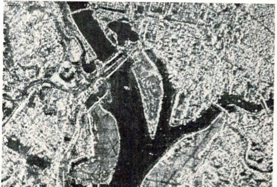
Map of Washington, D. C., made by AN/UPD-1 surveillance radar
