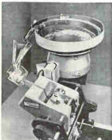
Bowl feed unit for axial lead components feeds into plastic hopper which handles a specific component size. It can be used as an input attachment on lead straightening, testing, orienting and taping equipment made by Universal Instruments Corp., Binghamton, N. Y.
