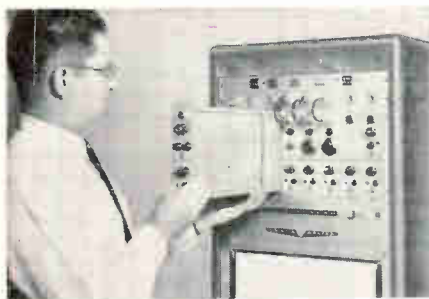
Entire channel easily accessible and completely interchangeable as single unit.
