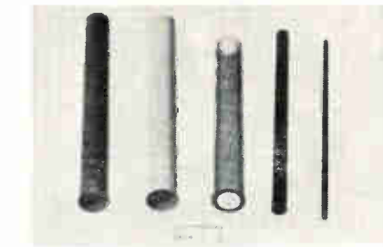
Epoxy tubing of various diameters and wall thicknesses (left). Component encapsulated in an epoxy tubing with an epoxy resin (right)
