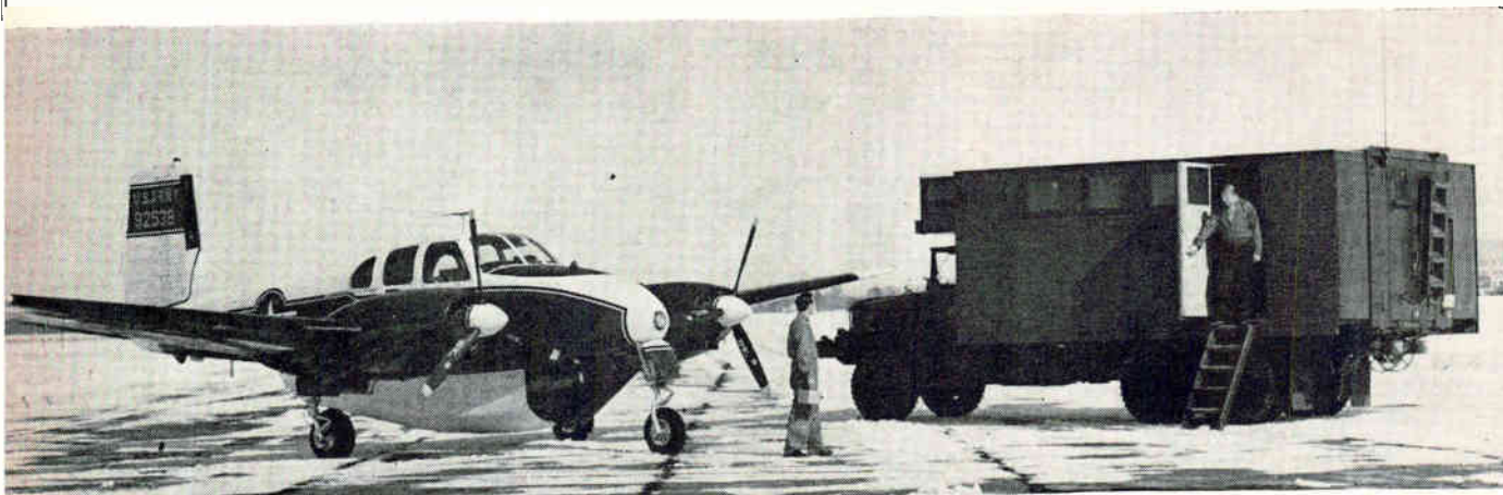
Radar operator delivers film from AN/UPD-1 radar plane to processing van
