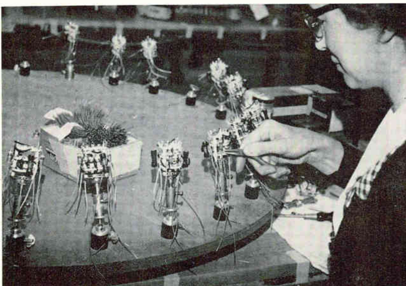
Standard camera tripod heads make a convenient holder for shafted sub-assemblies. The assembler can cock the head to the most convenient working angle. Sierra Electronics Corp., Menlo Park, Calif., mounts two dozen heads on a round of plywood to make a merry-go-round assembly fixture. The heads can also be used to mate subassemblies such as multipin connectors and rotary switches
