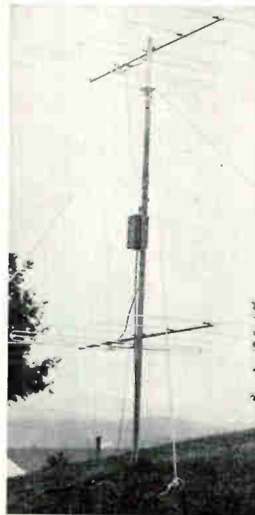
Five-element Yagi antenna on 21-ft mast for 1,000 microvolt per meter field-strength measurements, left, and antennas arranged for 200 and 40 microvolt reception at right
