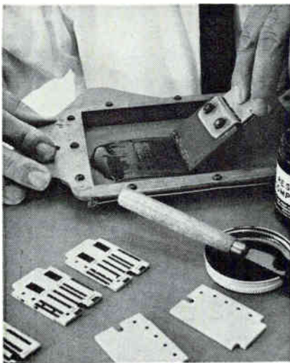
In laboratory demonstration, thin film of resistor composition is applied to ceramic base by stencil screen and squeegee (left). Stencil is removed from ceramic base leaving film of resistor composition ready for firing (center). Uses of new composition include ceramic printed circuits and resistor rods (right) where resistor paste is applied to a ceramic rod, fired and then spiralled to resistance value by a diamond wheel
