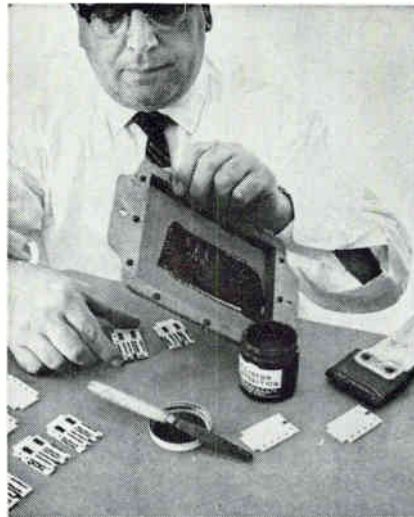
In laboratory demonstration, thin film of resistor composition is applied to ceramic base by stencil screen and squeegee (left). Stencil is removed from ceramic base leaving film of resistor composition ready for firing (center). Uses of new composition include ceramic printed circuits and resistor rods (right) where resistor paste is applied to a ceramic rod, fired and then spiralled to resistance value by a diamond wheel
