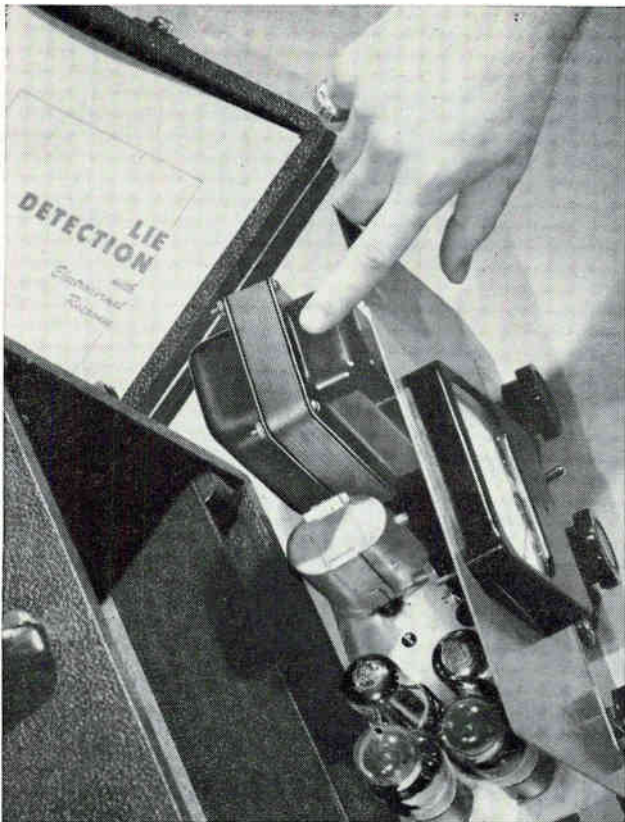
Above —Sola plate-filament transformer is built-in component of B & W Associates lie detector. It supplies plate and filament voltage regulated within \pm 3\% even when line voltage varies from 100 to 130 volts . . . helps assure accurate operation in field.
