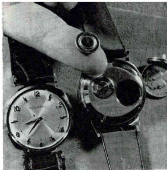
Hands are set by raising and turning the semicircular handle at the rear of the watch. The 1.3-v mercury cell, which lasts a year, is replaced by removing a cap that can be unscrewed with a dime
