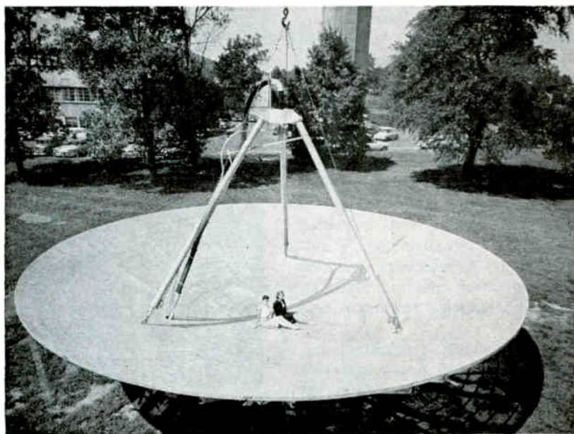
This 40-ft dish antenna at ITT will receive radio signals reflected from the moon or passive satellites
