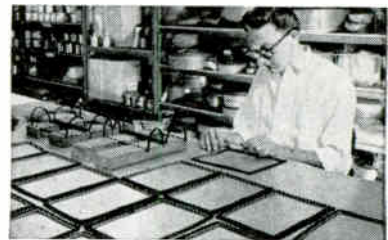
Rope is cemented to gaskets to form combination seals
