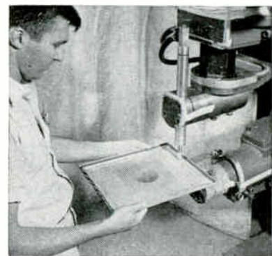
Aluminum holding strips facilitate welding to metal closures
