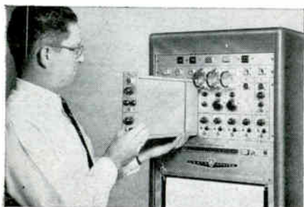
Entire channel easily accessible and completely interchangeable as single unit.
