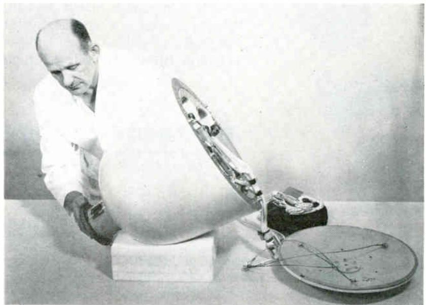
Nuclear emulsion recovery vehicle (NERV), by GE, was recovered after being launched to 1,200-mi altitude to measure radiation
