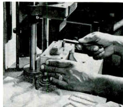
Small shielding gaskets are made by die-forming stockings
