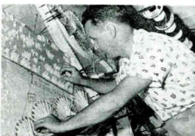
Section of board shown on cover. Harnesser is coding wire ends
