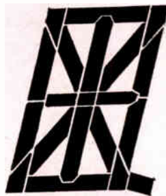
EL "READOUT" DEVICE is composed of strips of electroluminescent lamps, insulated from each other and separately terminated. By selective excitation of the "strips," alpha-numeric symbols are produced for readout purposes.
