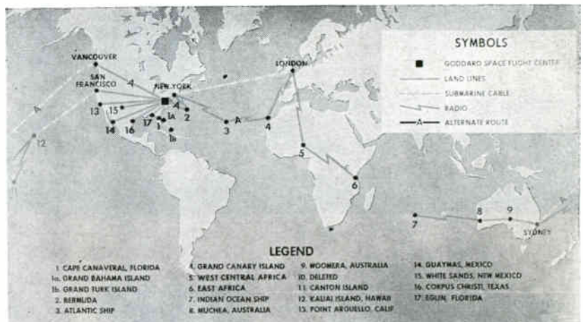
Ground communications use landlines, submarine cables and h-f radio
