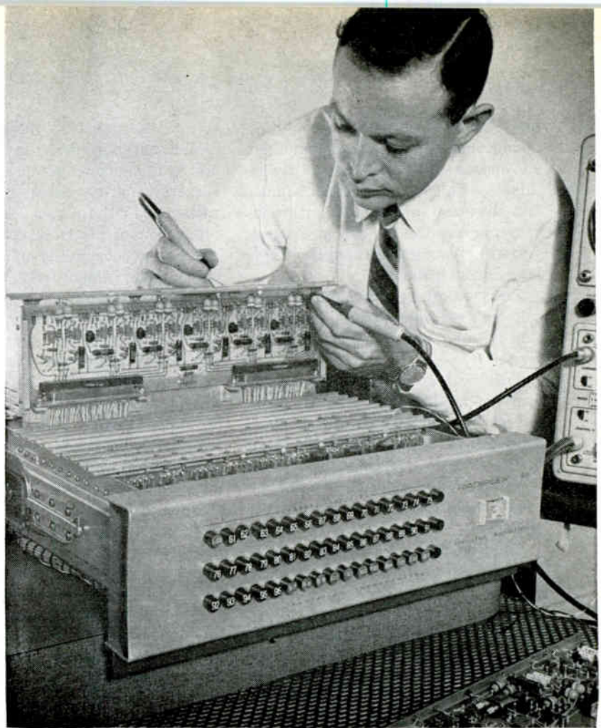
Electronic multiplexer can directly acquire and multiplex outputs of low-level strain gages, thermocouples and other transducers
