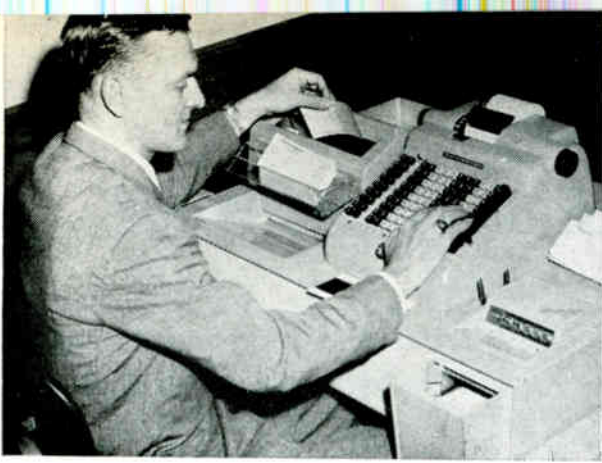
Burroughs account and amount imprinter (left) places magnetic ink characters on uncoded checks as first step in automatic processing. Sorter-reader (right) developed jointly by Pitney-Bowes and National Cash Register separates checks according to banks originating them by reading MICR code
