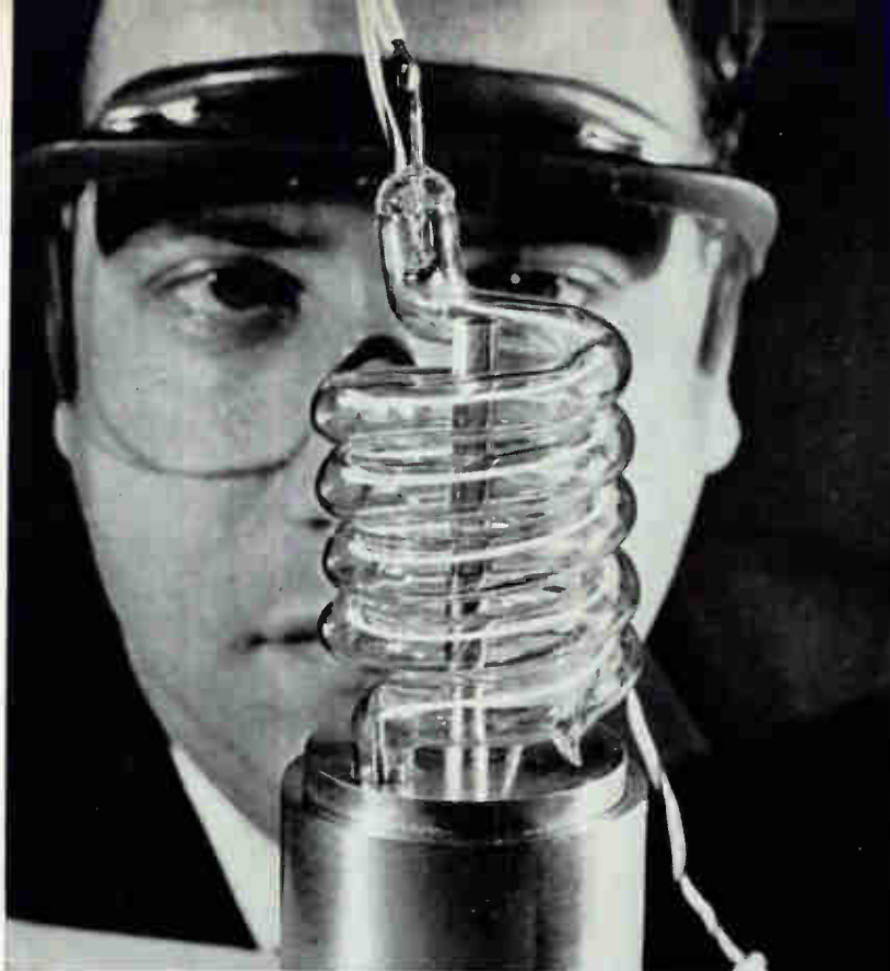
Synthetic rod-shaped ruby crystal sits in metal casing. Excitation energy comes from spiral gas discharge lamp
