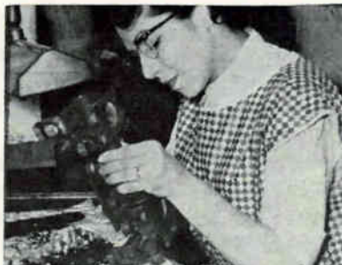
Gating system is wax-welded to the pattern
