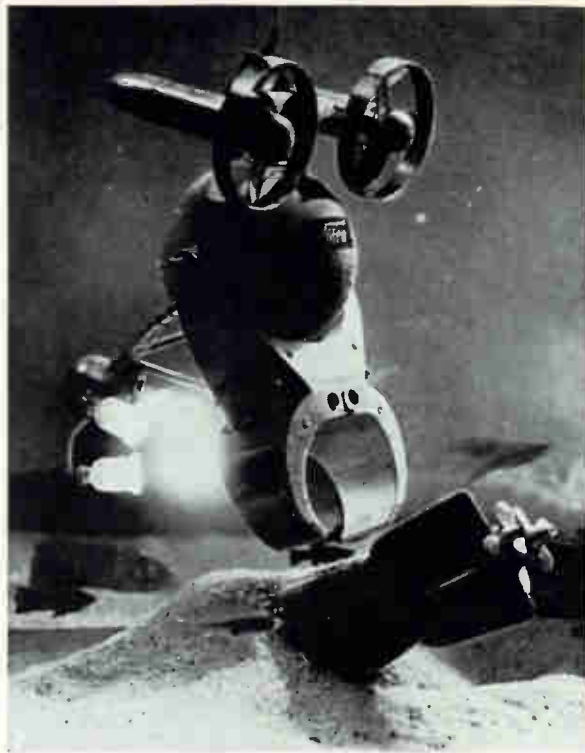
With its tv camera trained on the claw, this Solaris model gets into position to recover a torpedo
