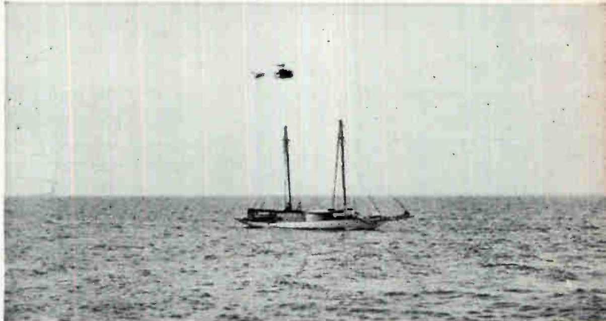
Schooner Azara carries the artificial lightning generator. Helicopter supports the 10,000-foot antenna
