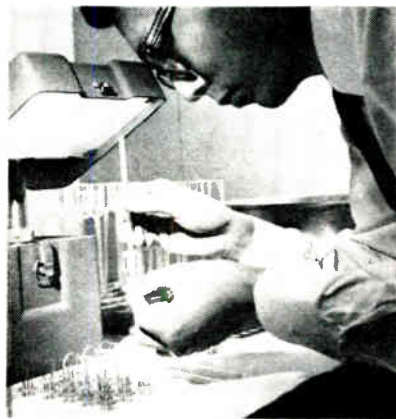
Fit between mating bulb and stem edges is indicated by fringes seen under monochromatic helium light
