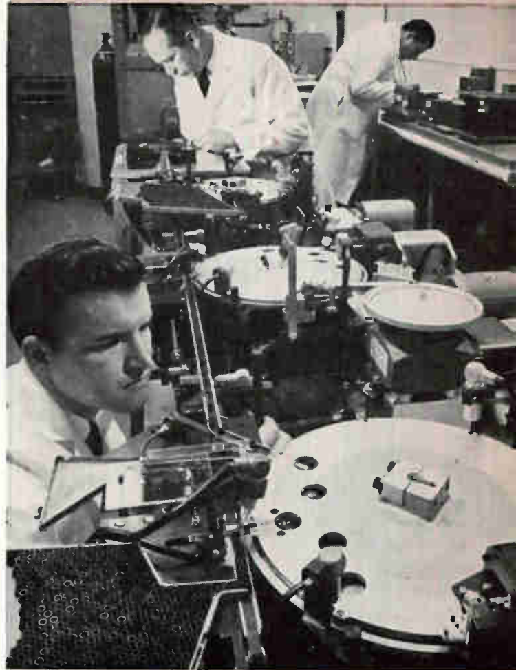
Fully automated transistor assembler. Carbon boats convey transistor components to assembly stations
