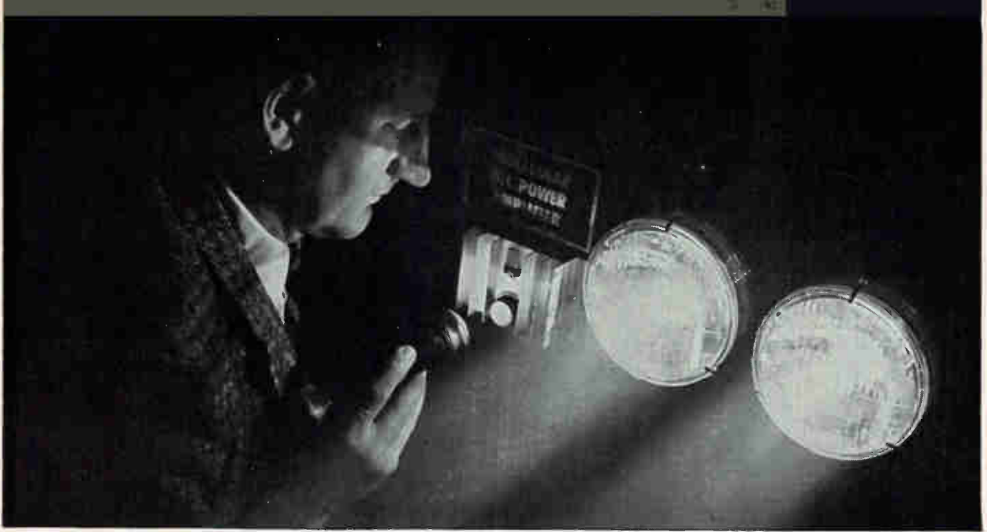
D-C AMPLIFIER: connected to a solar cell, this tiny block takes an input of 4 milliamps . . . via flashlight beam, raises it to 40-watt output.
