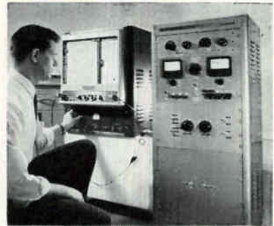
Output of instrument is fed to X-Y recorder to obtain magnetic characteristics
