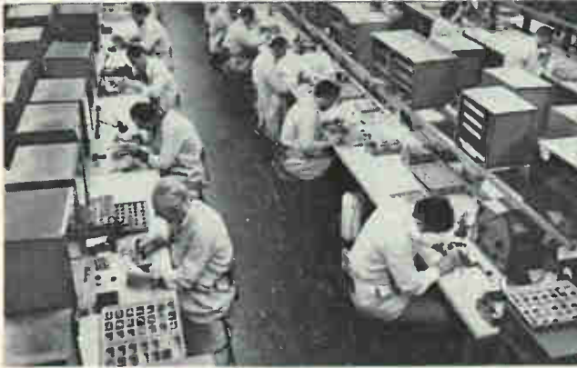
Trays with numbered cavities provide each assembler with a parts kit for a specific assembly or subassembly
