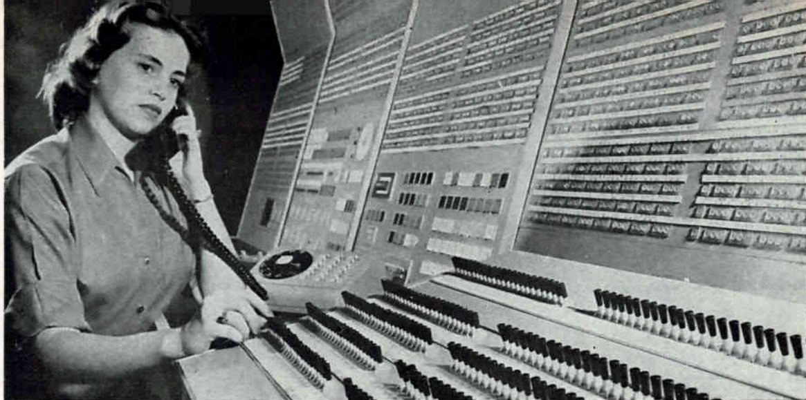
Mock-up of data processing subsystem console for SAC's new world-wide combat control system
