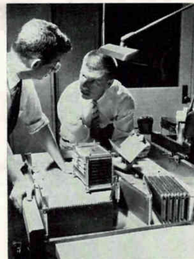
Basic components of the Twistor module are discussed by H. L. Stadler and D. G. Clemons of Bell Laboratories. Readiness for mass production was accomplished through the closely coordinated research-engineering work of Bell and Western Electric. A partially assembled module is in the foreground, with a completed unit behind it
