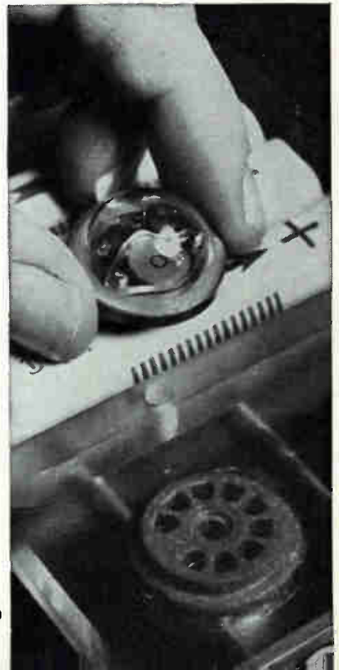
LIGHT TELEMETRY SUB-SYSTEM: a single light-responsive monolithic element delivers output whose frequency is a measure of light intensity.
