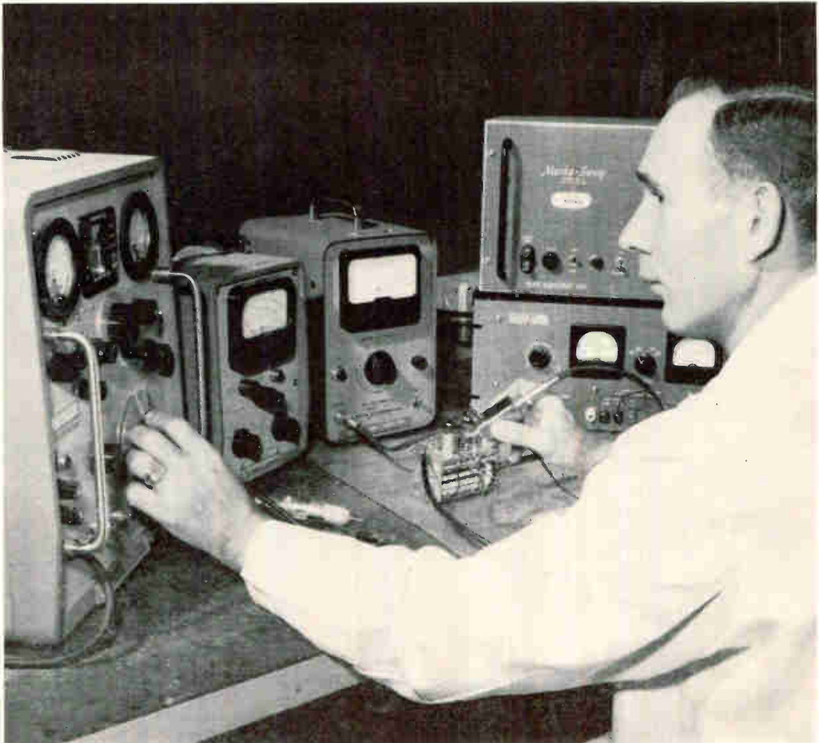
Measuring r-f output of modified turret-type tuner
