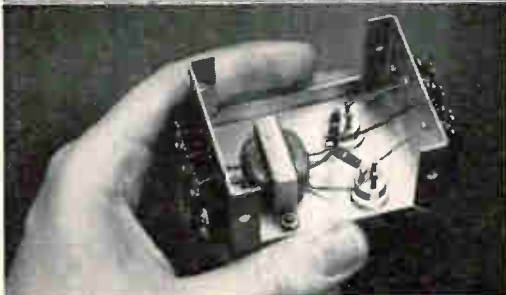
Compact, lightweight servo amplifier employing CBS 2N1434 10-watt push-pull output stage.
