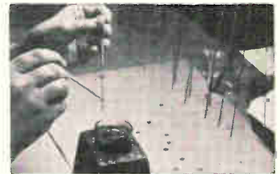
Bundle is primed with encapsulating compound
