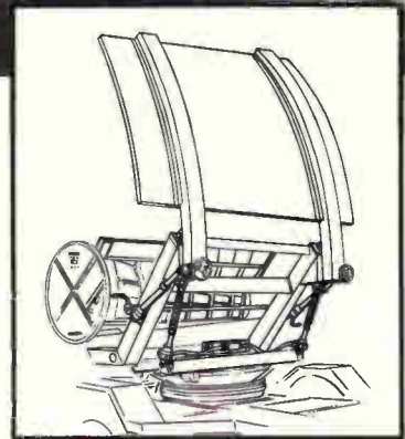
U.S. Army Signal Corps ground portable radar unit operated with two AiResearch electromechanical actuation systems.
