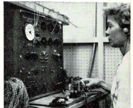
100% final inspection is made possible by this exclusive high-speed system developed by Bourns to test all major electrical characteristics. Critical dimensions of each unit are also checked.
