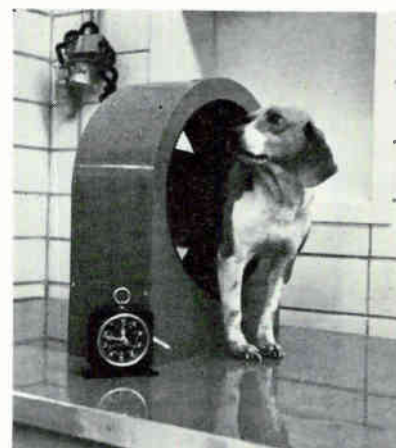
Suzie, affectionate beagle used in Smith Kline & French Laboratories' experiments, stands quietly—but a bit puzzled—in firm's new induction heating coil. Device, which is able to open capsules and release drugs at predetermined areas of dog's gastro-intestinal tract, enables scientists to study absorption of oral drugs without any direct electrical or mechanical attachments
