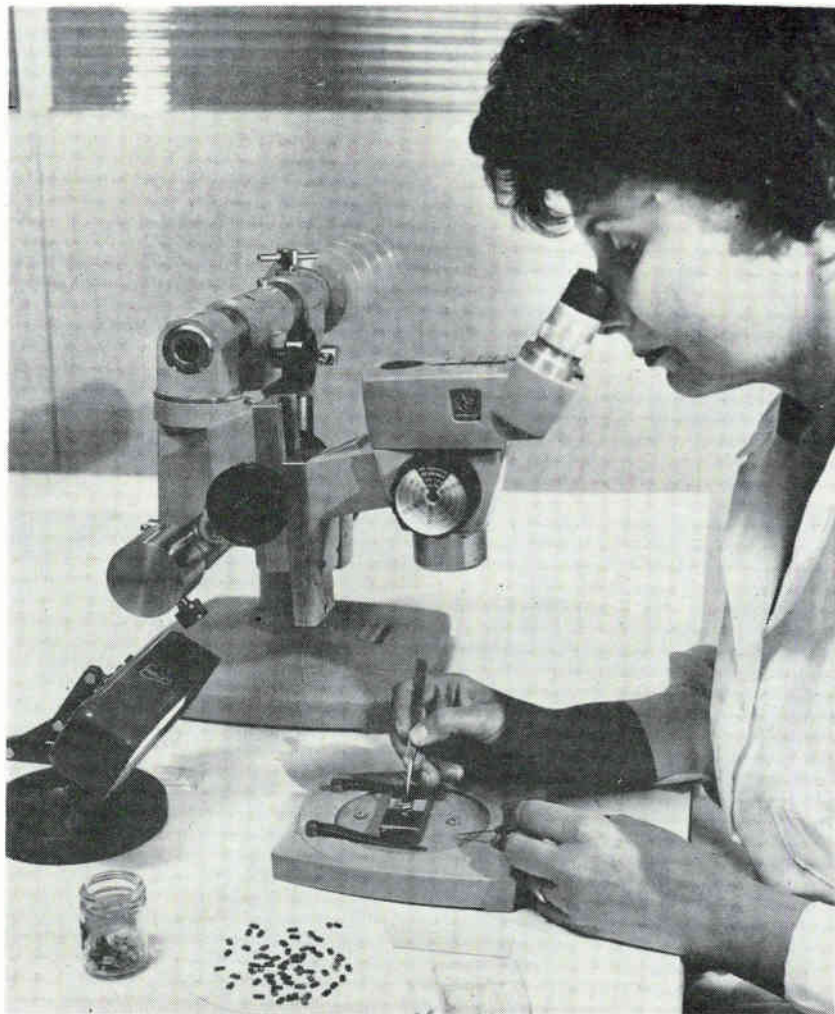
Technician at RCA inserts preproduction sample of tunnel diode into its miniature low-inductance case
