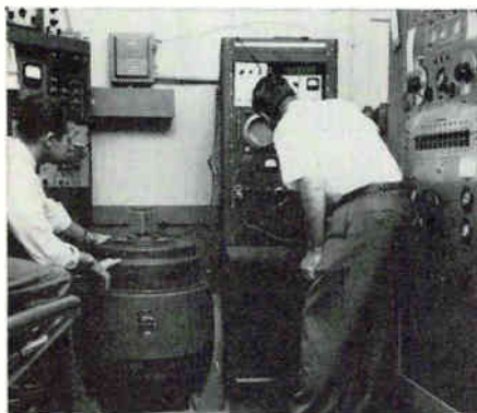
This vibrator for measuring conformance to Mil-Specs is an important part of the extensive equipment in Bourns Reliability Assurance Laboratory.
