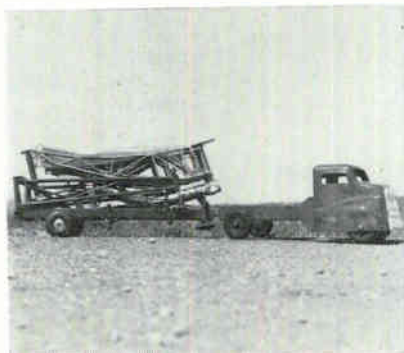
New tracking antenna, built by D. S. Kennedy, can be collapsed into a compact bundle and towed (left) by a light truck or station wagon to new site, then opened. System consists of a 28-ft folding, cloth-surface reflector, hand-operated elevation-azimuth drive (motors and selsyns can be added if desired), and a self-contained trailer mount and tower
