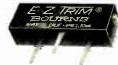
Low Cost Commercial Wirewound E-Z Trim—Model 277. Subminiature—1" x 17/64" x 5/16". Tapered all-purpose lug terminals / 1/2 watt / 100 ohms to 10K. For computers, test equipment, industrial control systems, etc.
