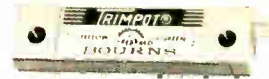
High-Temperature, Humidity-Proof Wirewound Trimpot—Model 224. Operates at 175 C / L,S,P terminals / 1 watt / 100 ohms to 100K. Meets Mil-Specs for humidity.
