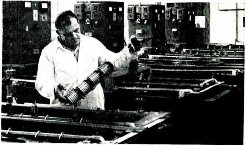
Machined plastic bodies of large ring assemblies are hung from oscillating rod
