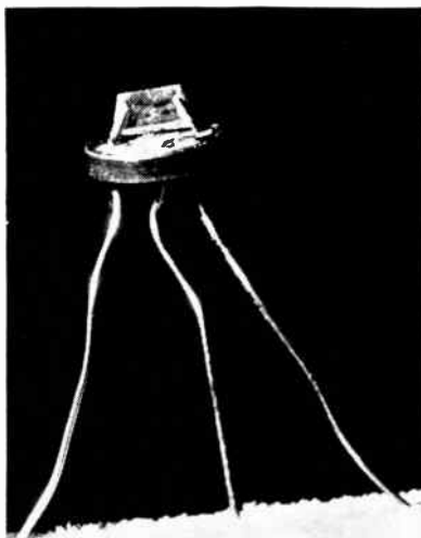
Esaki-diode oscillator mounted in a standard three-pin header. The outer pins are identical. Either one can be used with the center pin
