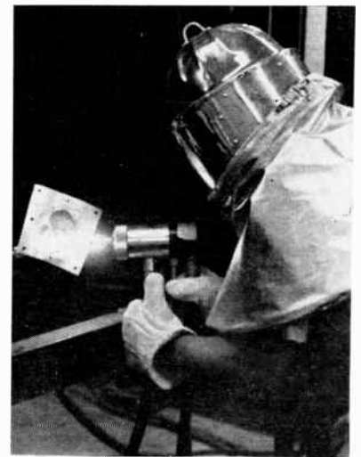
THE FRONT COVER. Antenna for tracking beacons in re-entry vehicle is subjected to arc plasma jet at Melpar, Inc. Tests determine if antenna at 1,500 C maintains constant electrical thickness, low dielectric loss and carbon-free surface. Other re-entry simulation uses require that arc plasma unit generate temperatures to 20,000 C, heat flux intensities to 1,800 BTU/ft 2 /sec and velocities of about Mach 2
