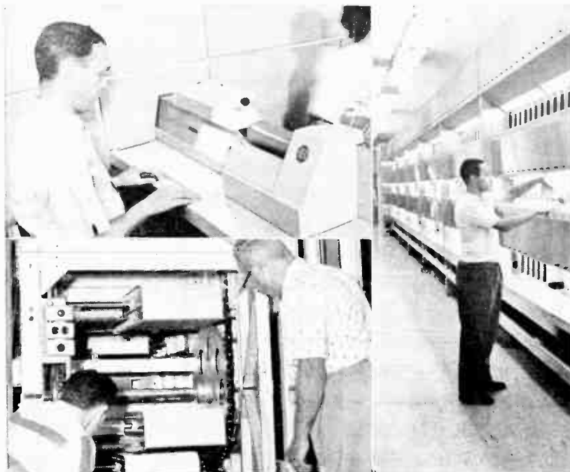
Photocell detectors and thyatron motor controls are electronics' contribution to postal mail-handling speedup now going on
