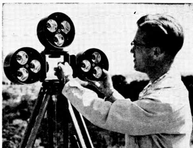
Geodimeter uses modulated light reflected from prisms to measure the distance between stations. Berg Hedstrom's model 4 unit shown here is portable with a maximum range of three to five miles and a minimum of fifty feet
