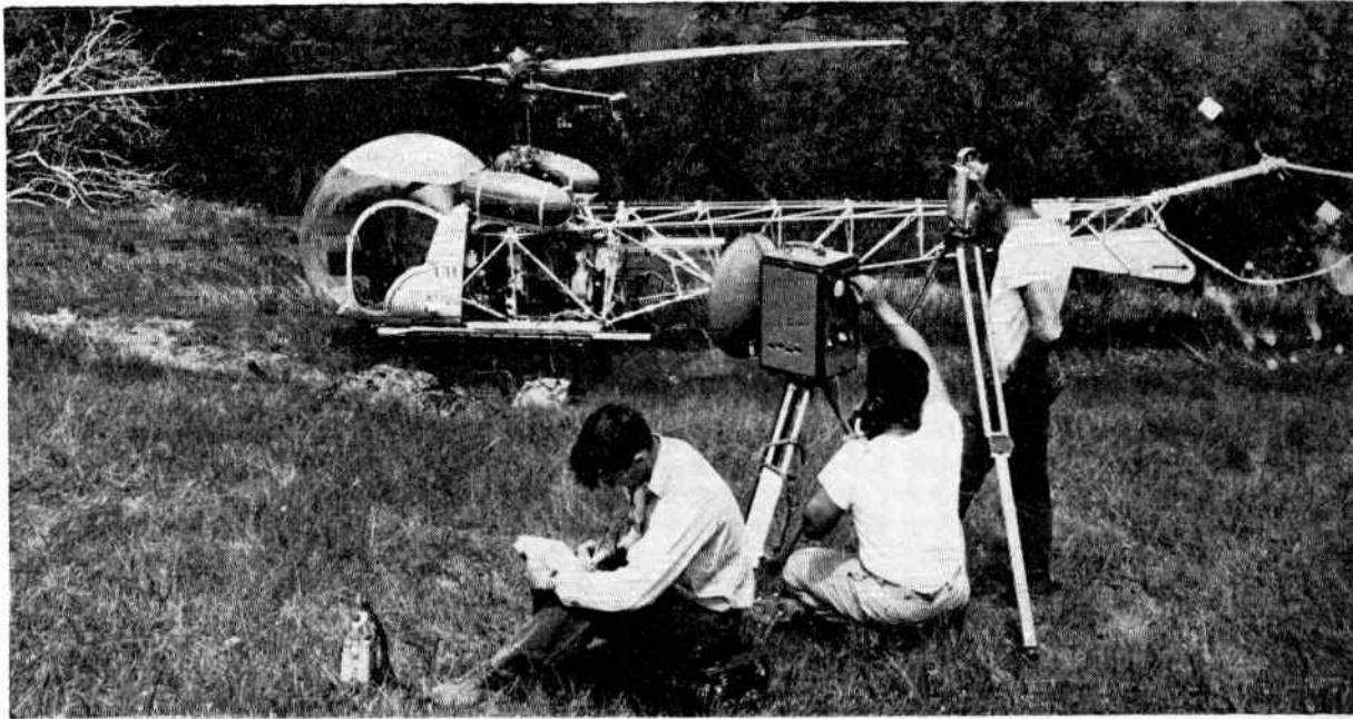
Eel River survey in northern California used a helicopter to transport microwave distance measuring equipment. Use of the instrument in the survey, conducted by California's Department of Water Resources, resulted in an estimated 50 percent savings. The helicopter made even further economy possible
