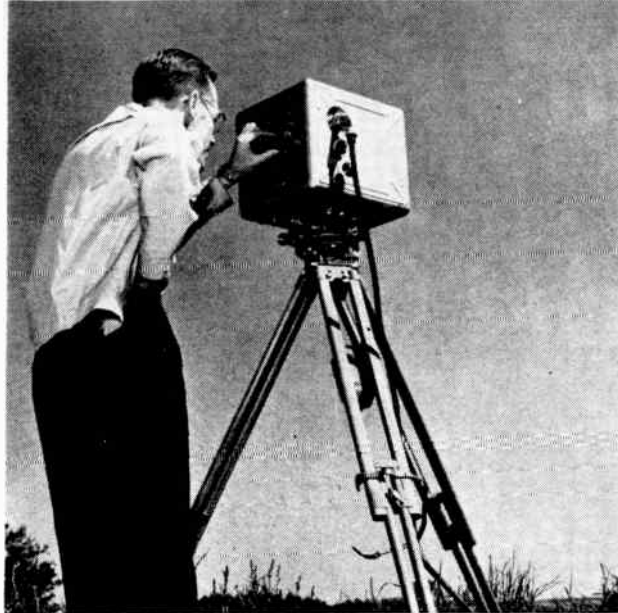
Geodimeter uses modulated light reflected from prisms to measure the distance between stations. Berg Hedstrom's model 4 unit shown here is portable with a maximum range of three to five miles and a minimum of fifty feet
