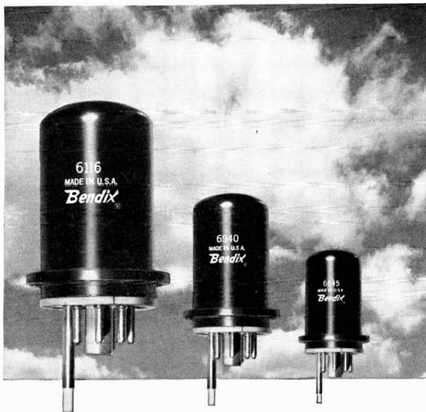
The 6116/TE-39 ruggedized Reflex Klystron thermally tunes a band of 8500 to 9660 MC by means of a diode within the vacuum envelope. Tuning speed over the required frequency range is 0.7 seconds min. to 3.0 seconds max.
