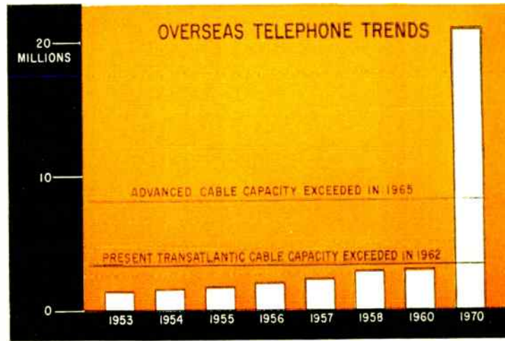
FIG. 1—Bar graph indicates that overseas telephone traffic is rapidly overtaking capacity of present and future facilities
