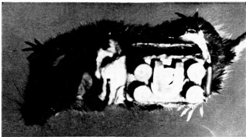
Visitors to 1959 International Trade Fair in Zagreb, Yugoslavia, saw radio-equipped mice in USAF School of Aviation Medicine display. Transistorized 20-gram unit transmits biological data to satellite telemetry system for retransmission to ground
