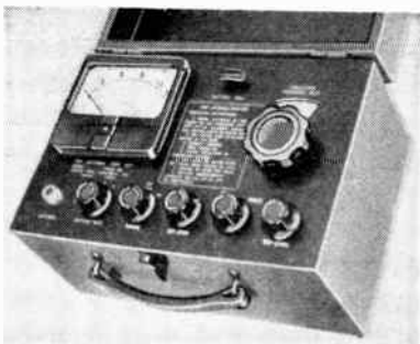
Meter is set to infinity with set level-read switch at set level (incident power setting)
