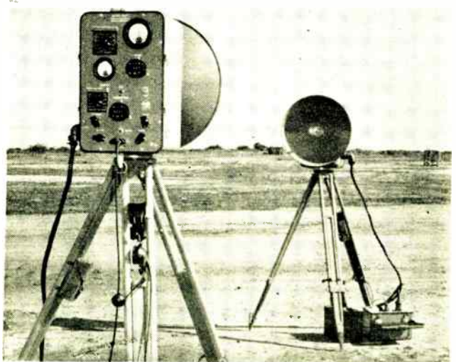
Micro-dist uses an r-f signal to measure distances. The two stations are interchangeable, one acting as an interrogator, the other as a responder. The time lapse between the original pulse and the return signal gives a measure of distance. Manufactured by Cubic Corp., the unit measures distances from 250 ft to 50 miles
