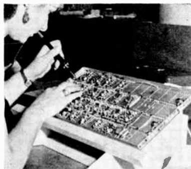
Lines of terminals are used as channels for hookup wiring
