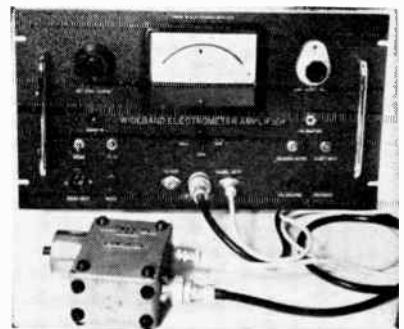
Electrometer stage V1 is inside a separate 5 × 3 × 2 in. screening box
