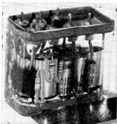
FIG. 1—Resolver drive amplifier shows application of 3-D packaging technique to analog circuits
