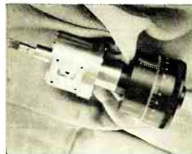
Wavemeter with a precision of about 3 parts in a million, developed by the National Bureau of Standards for accurate dielectric measurements
