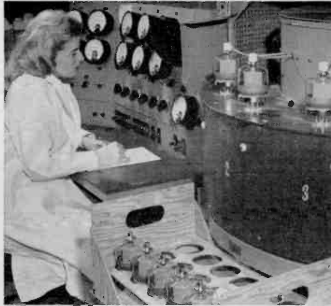
Every tube meets rigid Eimac specifications before shipment. On test consoles like this, dozens of electrical characteristics are patiently tested and recorded for each Eimac tube produced. Environmental testing equipment is also available for testing for severe applications.
