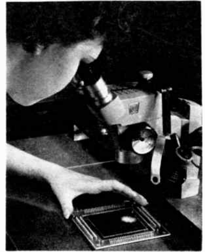
THE FRONT COVER. Production worker examines memory plane using ferrite memory cores for possible flaws
