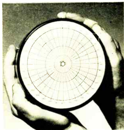
Interference with precise readout position on crt from parallax is eliminated by applying scale to inside face of tube
