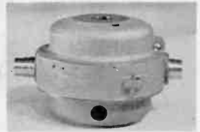
Completed assembly. Pivots are brazed to Monel body
