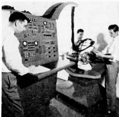
Test console and rate table, built by Amelco, Inc. for Douglas, makes all dynamic measurements necessary to evaluate the Inertial Guidance Flight Controller prior to its installation in the Thor IRBM
