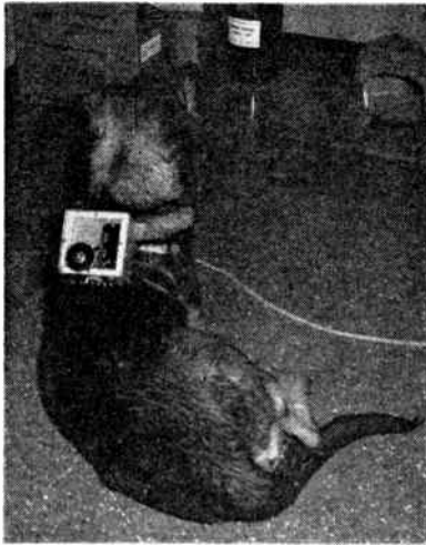
Battery-operated heart pacer in small package can be mounted on harness of test animals
