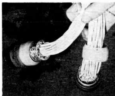
Old method (left) and new. Formerly all shields and the ground wire were soldered to common points. New technique grounds shield compactly, economically
