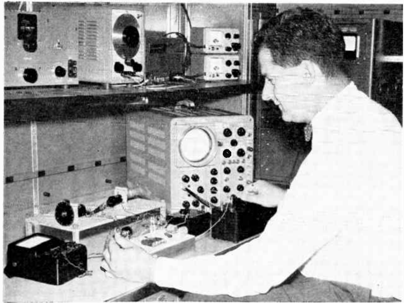
Engineer tests the wave shape, frequency and distortion of an experimental low-frequency sine-wave generator
