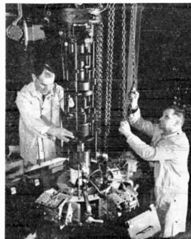
Multi-million watt klystron is being placed in new Sage radar system. The tube, developed jointly by GE and the Air Research and Development Command's Rome Air Development Center, will produce hundreds of times more power than the radar used to beam pulses to moon and back in 1946
