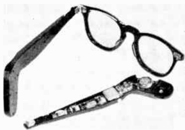
Antenna occupies entire left temple piece while radio occupies other temple piece
