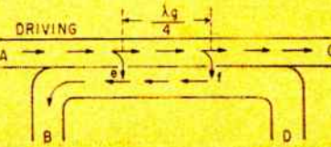
Signal path through orifice f is twice hole spacing longer than signal through e. The vector addition is zero
