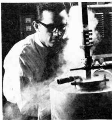
Absolute zero within 1 deg F is achieved by Sperry Gyroscope Co. scientist in tests of components for countermeasures systems. Equipment is being tested in bath of liquid helium
