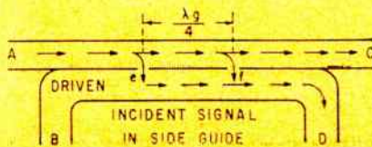
Signal through orifice e and f travel same path length, therefore add directly. Signal at D proportional to signal at A
