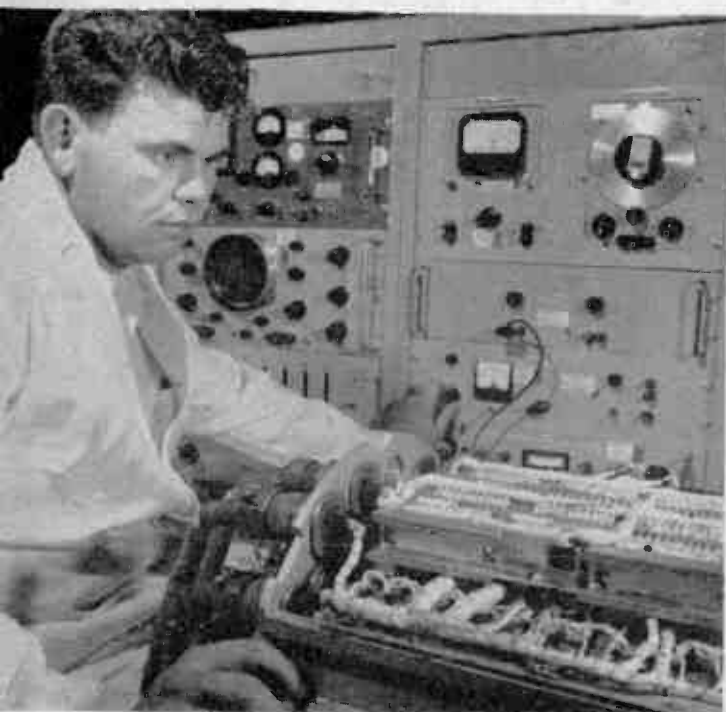
Instrument complex used to check out telemetering packages of Polaris test vehicles at Lockheed's Missiles and Space Division
