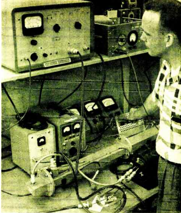
Engineer makes adjustments necessary to optimize noise figure within a system using Hewlett-Packard's noise-figure meter
