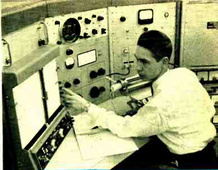
Operator checks out traveling-wave tube using automatic production tester built by Sperry Microwave Electronics
