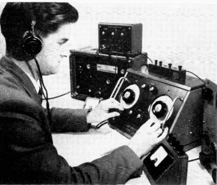
High-frequency transistor parameters are measured using Wayne Kerr r-f bridge
