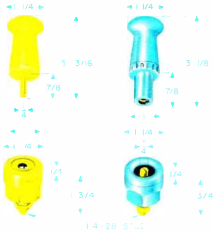
REQUIRE 1/4" PANEL HOLE 1/4" MAXIMUM PANEL THICKNESS 50 AMPERE TYPES
