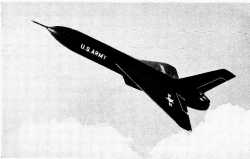
Army's SD-5 surveillance drone, now under development by Fairchild Engine, will carry a wide variety of electronic sensing devices
