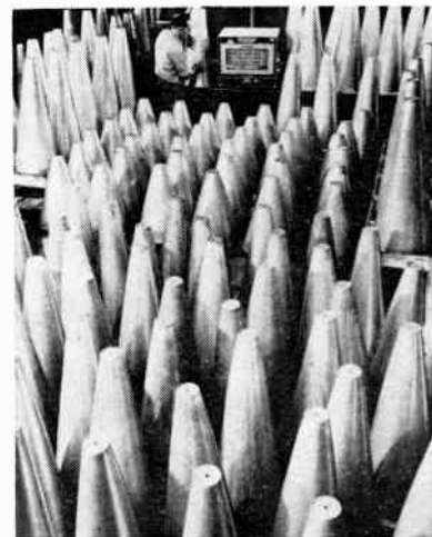
Nose cones for the Nike-Hercules missile here await inspection by use of an ultrasonic resonance gage made by Branson Instruments of Stamford, Conn. When the transducer is placed against the outside surface of the cone, high-frequency mechanical vibrations are transmitted into the metal. Fed back into an electronic circuit, resonant vibrations are shown by two or more vertical traces in the face of a cathode-ray tube. A scale indicates wall thickness directly. Wall thickness must be held to within \pm 0.006 in.
