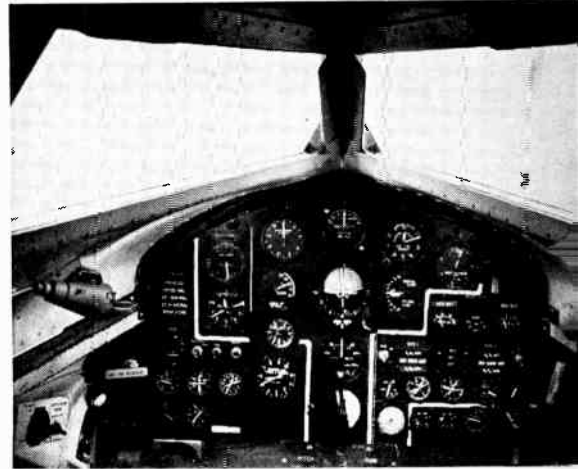
X-15 instrument panel showing the inertial speed, rate-of-climb and altimeter indicators (grouped at top right of panel)
