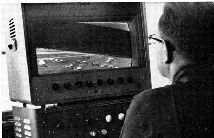
Closed-circuit tv at Atlantic City, N. J. airfield provides 7 by 3 aspect ratio picture. Developed by Grimson Color, Inc., monitor presents almost twice the information displayed by standard 4 by 3 aspect ratio screens
