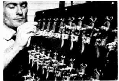
Test board holds 28 transistors. Rubber patches insulate toggles
