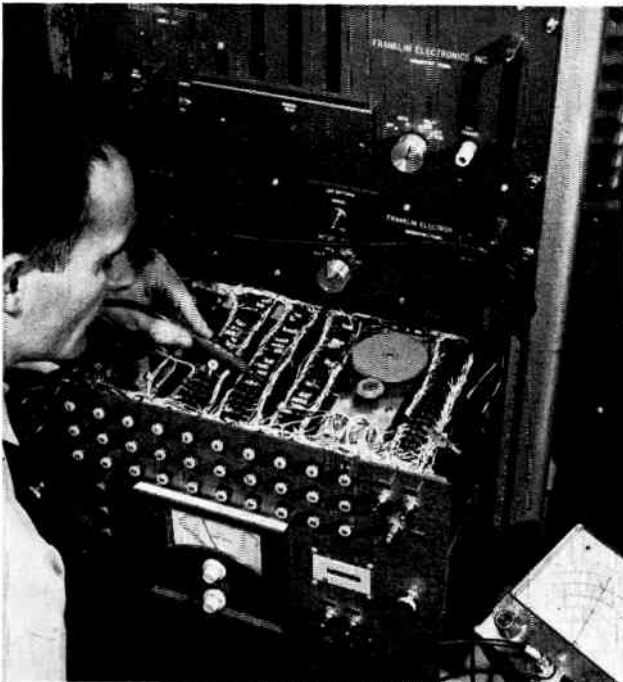
Control unit of sequential analyzer. Lights in horizontal rows indicate transistor under test, lights left of meter indicate test being made
