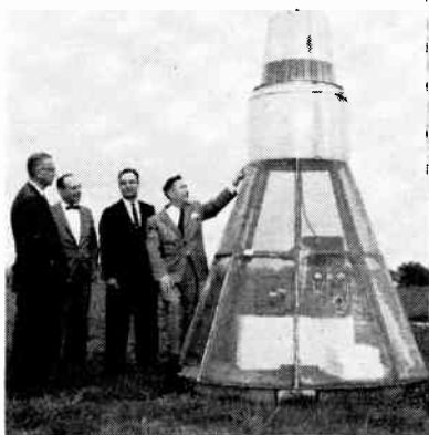
Full-scale antenna test mockup of Project Mercury capsule is being used in developing communication systems for the manned space capsule. Systems, designed by Collins Radio, will aid in putting such a capsule into orbit and recovering it
