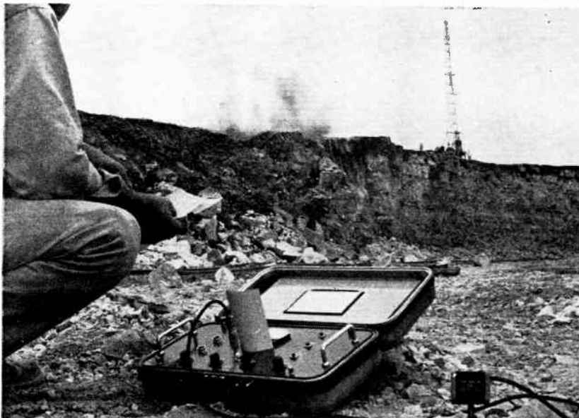
Battery-powered, portable Blastcorder by Geotechnical Corp. has fixed scale for immediately measuring peak accelerations from 0 to 1.1 g's. Device, usable with one, two, or three pickups, weighs 20 lb and provides permanent record on 4 x 6 transparent film
