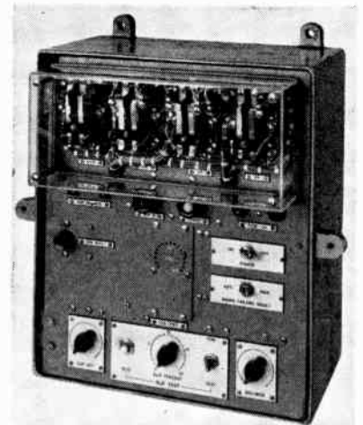
Conveyor guard unit with cover removed
