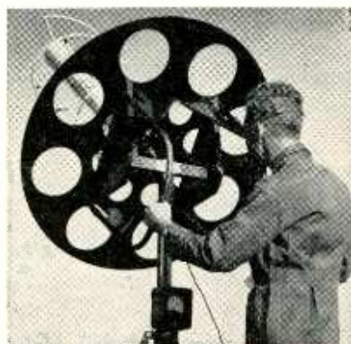
THE FRONT COVER.—Helix antenna picks up airborne transponder signals indicating distance between target and missile
