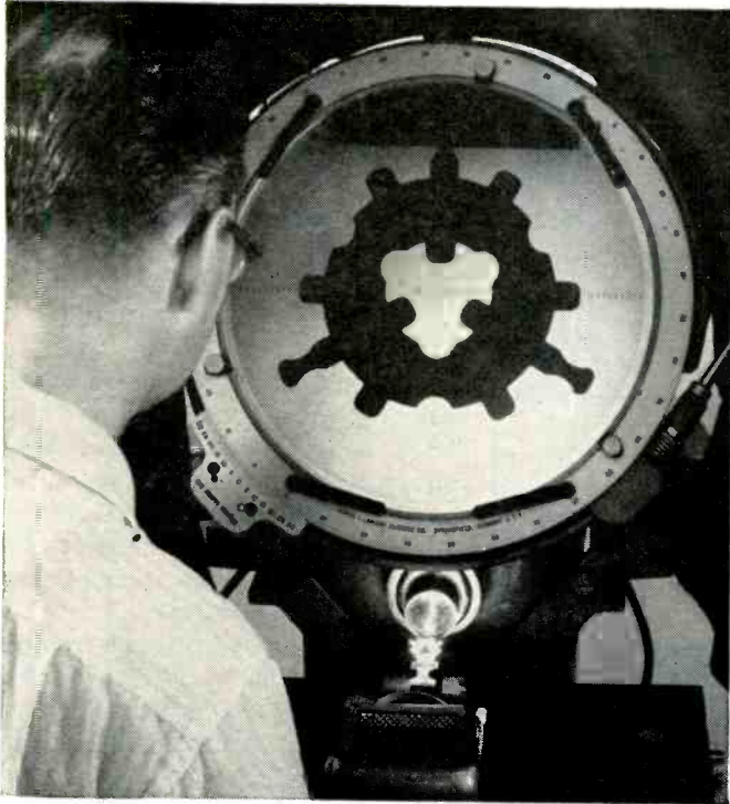
checking the critical dimensions of an armature commutator
