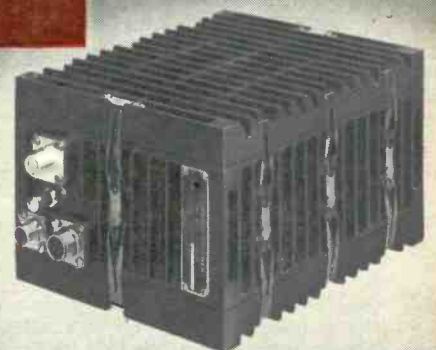
Weighting only 12 pounds, Crosley Command Receivers direct destruction of off-course missiles, control drone recovery.
