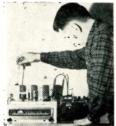
Tuning heterodyne adapter to desired subcarrier of f-m transmission. Heterodyne adapter couples to multiplex outlet of any f-m tuner
