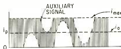
FIG. 2—Class-A amplifier plate current with auxiliary signal added
