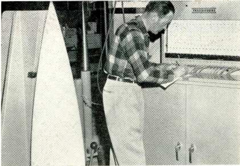
Thickness of radome at 23 points is read from position of metal floats positioned by air pressure. A total of 184 points is measured by rotating the radome
