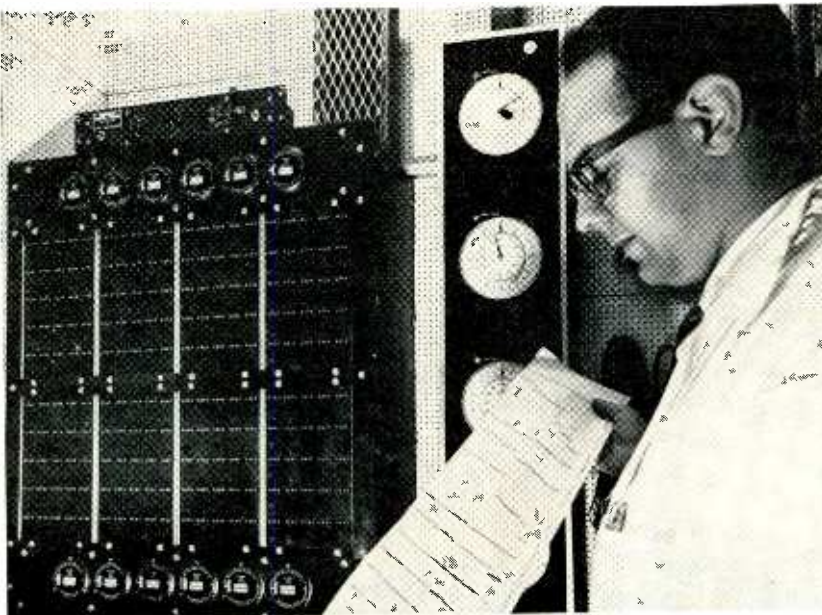
Performance of animals after being given new drugs is graphically recorded at Schering Corp. behavior laboratory. Landis & Gyr impulse counters show statistical pattern of behavior for comparison with behavior of same animal without drug
