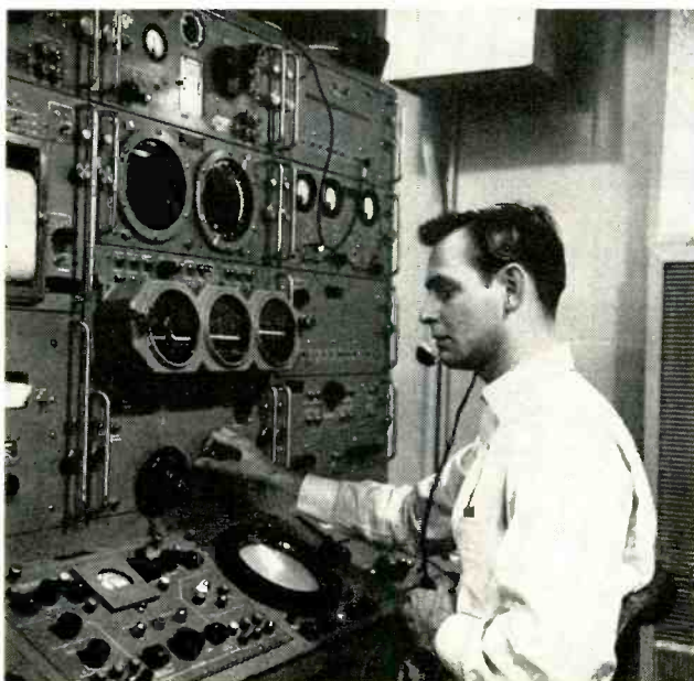
Console of Mod II radar. The set is an updated SCR 584, presents polar coordinates in both analog and digital form
