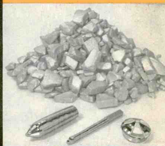
Three characterization crystals are grown from each lot — one for resistivity, type and lifetime determination; another for cleanliness; a third for boron content.
