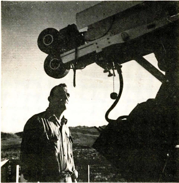
Boresight camera on AFMTC Mod II radar minimizes tracking errors by permitting calibration through comparison of optical and radar information
