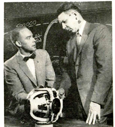
Heart of inertial system to guide nation's first man in space is examined by an engineer and (right) President Carl A. Frische of Sperry Gyroscope, which developed system. This stable platform uses miniature gyros and accelerometers which feed data to computers and instruments needed to guide space vehicles
