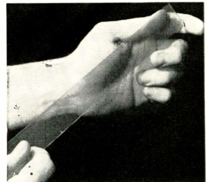
Typical strip of nuclear emulsion on glass backing used in cyclotron
