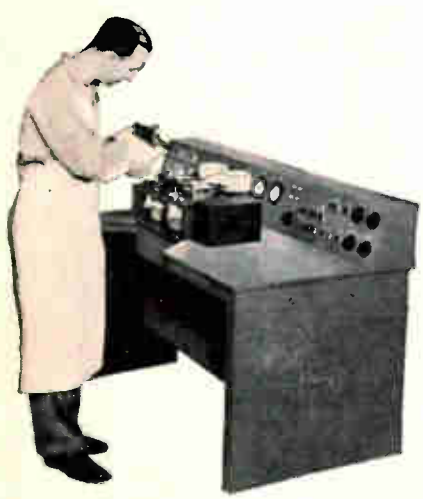
TI-designed fully automatic wafer sorter. Silicon wafers for TI diodes or rectifiers are vibration fed to pick-up stations where they are vacuum gripped by upper contacts of test arms. During transit to drop chutes, lower contacts are applied, polarity checked, test circuits adjusted, and tests performed . . . at a rate of more than 4000 per hour.
