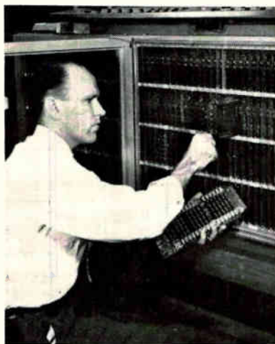
Compact circuit cards in Philco S-2000 characterize hardware in new transistorized computers
