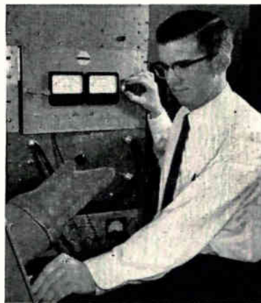
Adjusting channel width. Chronotron is device with two meters on front panel
