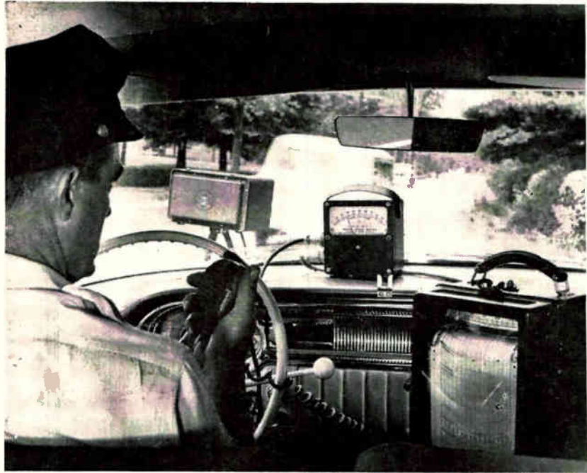
FRONT COVER. Radar speed meter mounted on tripod at roadside measures speed of passing car. Inside police car direct reading indication of speed in mph appears on meter while permanent record is made on strip-chart recorder
