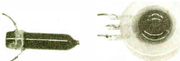
Typical solion units. At left is a visual readout integrator; at right, a linear detector
