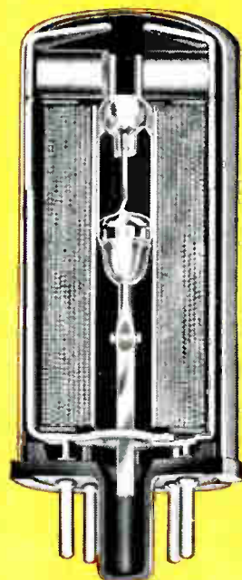
Cutaway view of a CLARE Type HGS Relay. Mercury-wetted contact switch is sealed in glass and surrounded by the operating coil. Biasing magnets are attached to the upper ends of the side plates.
