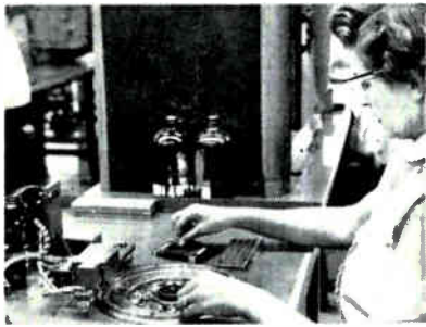
Operator color-codes cases with ink pod as she removes them from turntable
