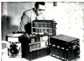
The completely transistorized RW-30 airborne digital computer has a volume of 4.19 cu. ft. and weighs only 203 lbs., including power supply
