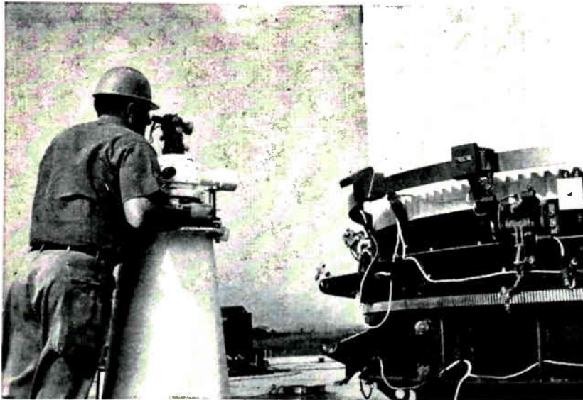
FIG. 1—If monitored mirror is not perpendicular to line of sight, modulated light reaches multiplier phototube
