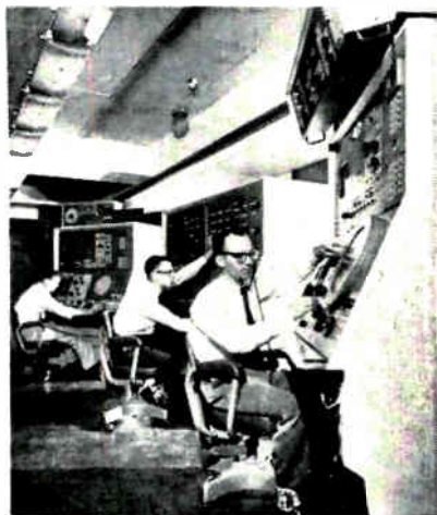
Plotting and recording gear (left) is among equipment RCA installed and will operate on S. S. American Mariner, new "missile measurement ship" now active on the Atlantic Missile Range. Huge dish is described as largest tracking radar antenna afloat
