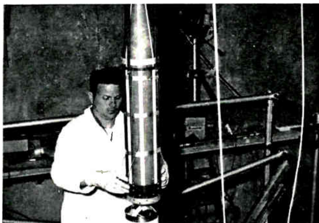
At left, engineer prepares part of instrument package for shake table test. During power phase of launching period, payload was exposed to a force of approximately 100 gravities. At right, assembled payload is lowered onto fourth-stage rocket motor, the culmination of 80 days of intensive effort
