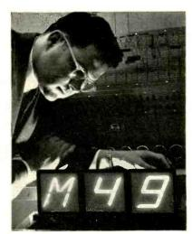
FIG. 8—Demonstration model of Westinghouse's electroluminescent lighting display system
