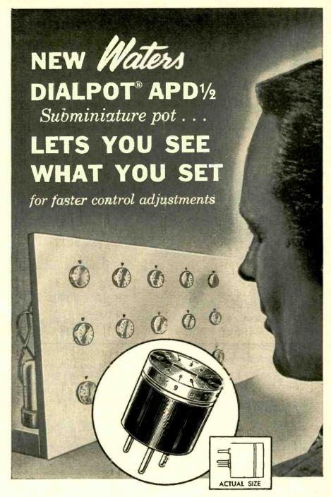
Plugged into printed circuits or mounted on control panels, this new ½" pot speeds adjustments by letting you see what you've set. Its dual-calibrated dial tells at a glance slider location, shaft angle and voltage percentage. The 300° winding angle is equally graduated from 0 to 10. Zero on the dial lines up with a scribe line on the side of the pot at 0° rotation. Terminals are located on a standard 0.1" grid, as used in printed circuits.
