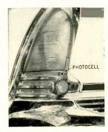
ing vehicle which is a great distance away, the 400-cps warning signal is of low intensity, indicating a moderate degree of collision danger. As the closure distance decreases, the warning signal becomes louder, indicating a more dangerous situation. A scheme for using lights to indicate less hazardous conditions and an incessant, imperative sound to warn of critical conditions is being studied.
