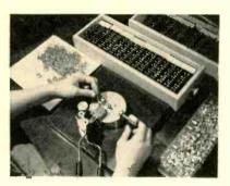
Jig bends leads of diodes into position
