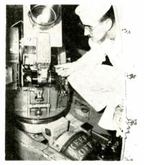
Electronics technician adjusts camera assembly of Fairand's photoelectric sev tant now being evaluated on USS Compass Island. Sensing device is image orthicon tube
