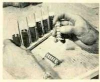
Fixture holds 6 resistors in Teflon for easy parting after cure
