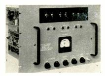
Digital timing generator generates reference time base, records time in hours, minutes and seconds on magnetic tape and displays time information in Arabic numerals
