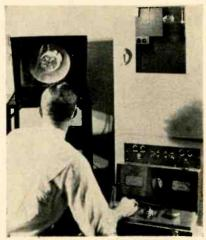
Industrial image amplifier enables x-ray inspection of devices with moving parts. Above, Picker X-Ray Corp. shows how its system would be used to inspect a gear. The television monitor permits remote viewing
