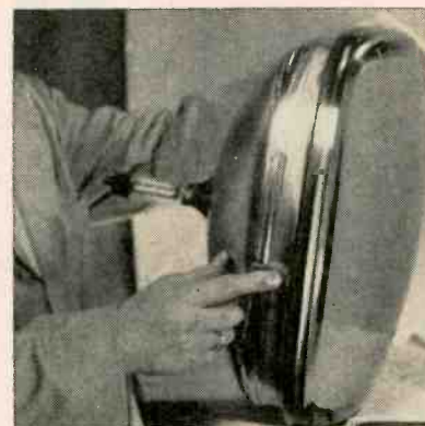
After cure, plastic has formed permanent seal between tube and panel
