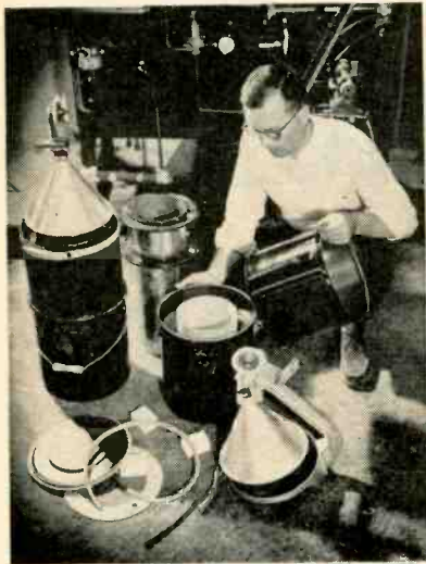
Inner and outer pail extensions guide wire into cone of dereeler
