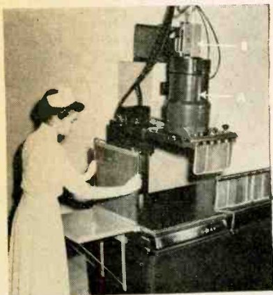
New image amplifier (A) for x-ray equipment is readied for operating demonstration with closed-circuit tv camera (B)
