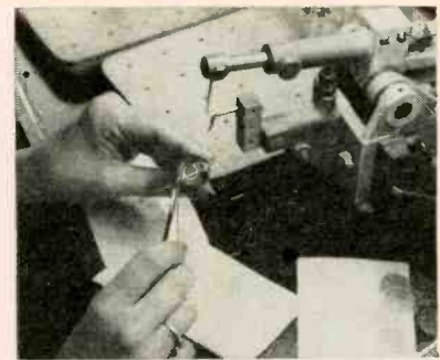
After characters are stacked projecting tabs are bent to pins and welded
