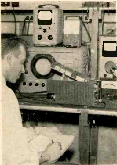
Design engineer checks crystal reference system for the 920 channel vhf f-m receiver-transmitter
