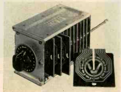
Typical communications switch illustrates simple method for inserting rotary-switch wafers. Removed wafer is at right
