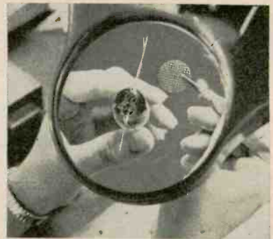
Placing anode screen on top of stack completes mount assembly
