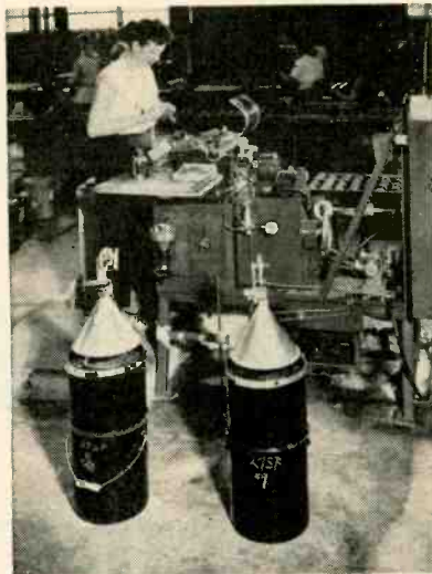
This setup supplies 300 feet of wire per minute to 2-pole motor winder
