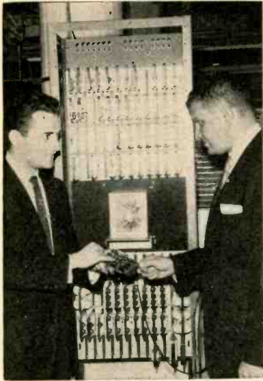
Memory rack—Apertured ferrite plate is used as memory or switch
