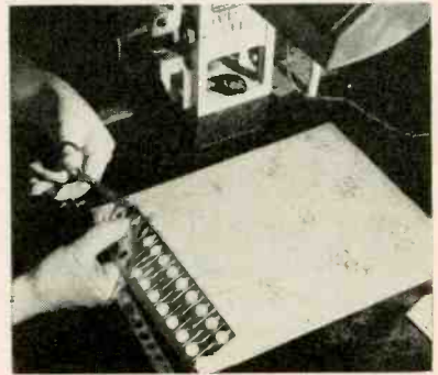
Photo-etched characters are cut from protective frames
