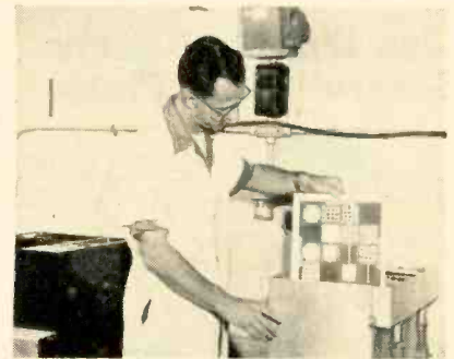
Etched board is washed in rinse tank
