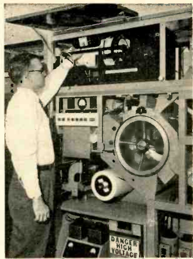
Operator is shown checking final adjustments prior to actual operation of the high-speed electronic printer. The character-forming tube is in the top panel
