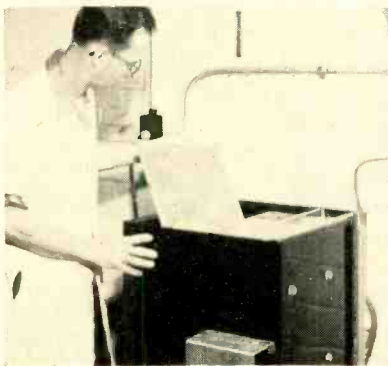
Unetched board is inserted in paddle etcher
