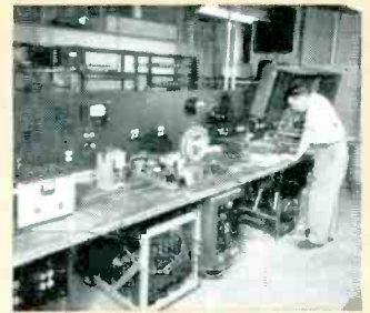
This power panel provides AC or DC in a wide range of currents, voltages, and frequencies . . . permits testing Ohmite products under operating conditions.
