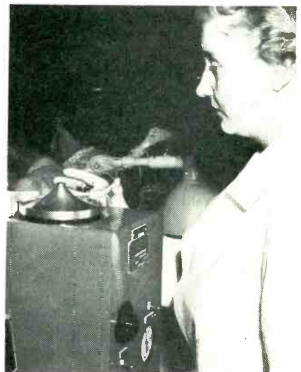
Transferring germanium pellets from watch glass to input cone of work feeder
