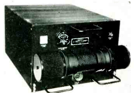
Transmitter used to send television observations from aircraft traveling at supersonic speeds
