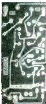
COMPACT CHASSIS BOARD USED IN SONIC INDUSTRIES' TWIN SPEAKER PORTABLE HI-FI PHONOGRAPH. SPACE AND WEIGHT PROBLEM REDUCED TO A MINIMUM WITH "THRU-CON".
