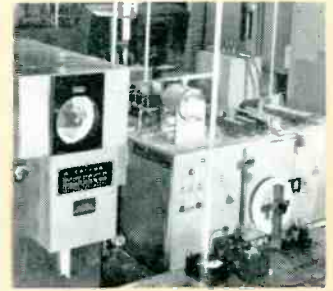
Humidity chambers using program-controlled cycles; here Ohmite products are tested under a wide range of temperature and humidity conditions.
