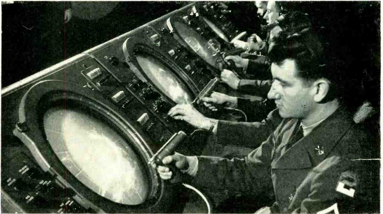
Thirty-target radar simulator is used in training personnel for the Army's Missile Master computers. These operators use photoelectric light guns placed against display console to enter targets in electronic tracking system
