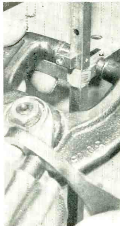
Appearance of joint after crimping. Pivoted block on left jaw of crimping tool is attached to washer for free rotation, to give precise positioning of dimple in center of tubing for any working angle of tool
