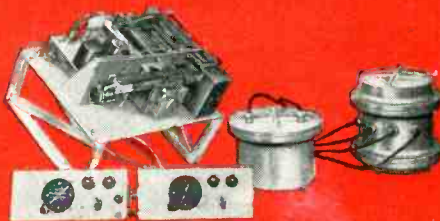
Underwater Servo Control System
