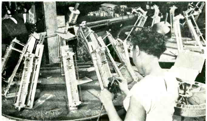
Assembling i-f terminal boards on single-operator turntable. Bent upper part of turntable shaft supports solder spool. Molded plastic rotating tray on floor stand at right holds needed components. Job card book above tray has one instruction card for each component to be installed
