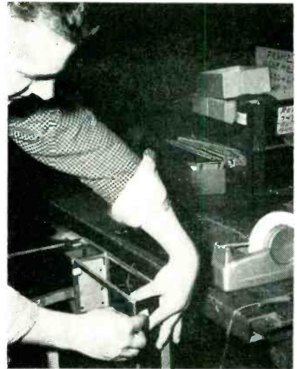
Holding woven aluminum bonding over tubing with masking tape, in preparation for riveting panel into position on frame for airborne jammer
