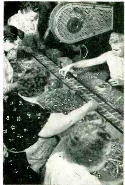
Color-coded conveyor setup used in final assembly of cam and locking lever on slide. Conveyor brings assemblies to press operator at left rear
