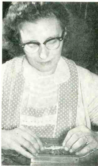
First step in assembling slide for cam-and-lever type auto radio pushbutton tuner involves loading two parts into pass-along fixture
