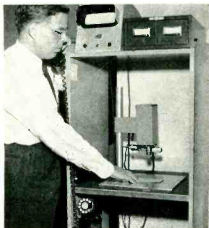
Data sending (left) and receiving (right) installations in Philadelphia bank of slow-sweep tv using telephone-company lines
