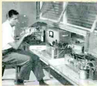
Instruments shown above are used to check and standardize the many pieces of Ohmite electrical test equipment.
