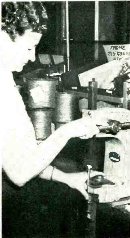
Holding tubing in position on adjustable stop of arbor press, in preparation for driving fitting into end of tubing
