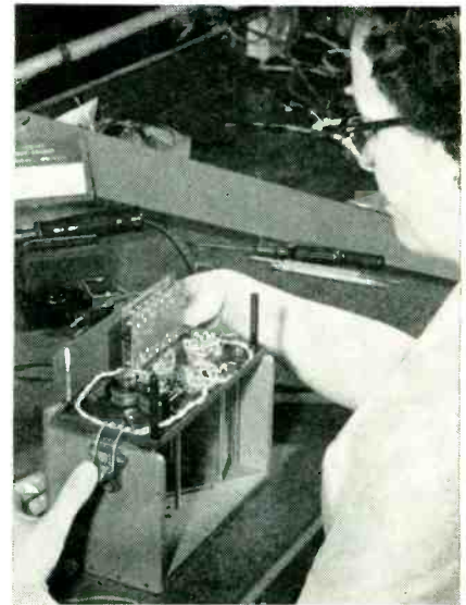
Pushing down luggage clip to anchor chassis on holding fixture
