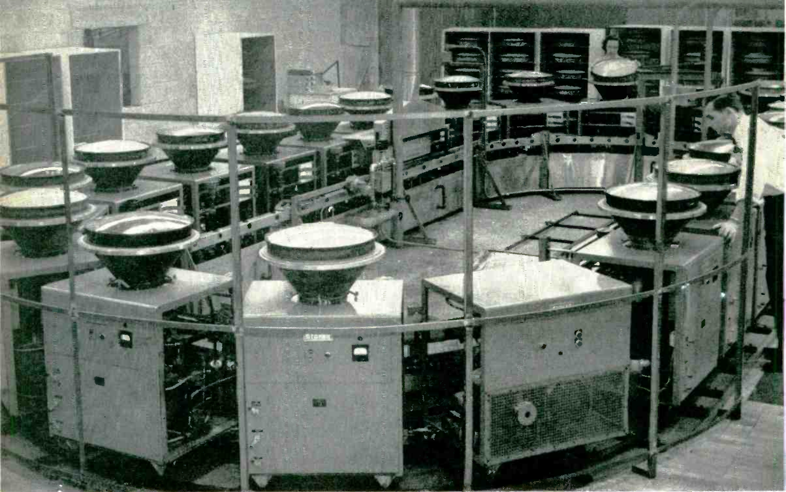
Automatic production at high output per man-hour is obtained from this complete in-line Stokes aluminizing system, used for color TV tube face plates at the RCA tube plant, Lancaster, Pa.
