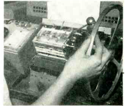
Operator sets large dial scale to desired new angular position with right hand and adjusts bridge with left hand to calibrate completed capacitor within tolerance of 0.02 micromicrofarad
