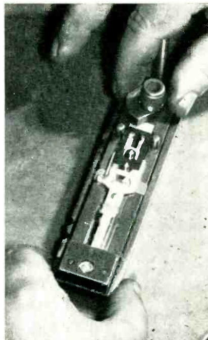
Turning hold-down cam after placing black locking lever spring over slide
