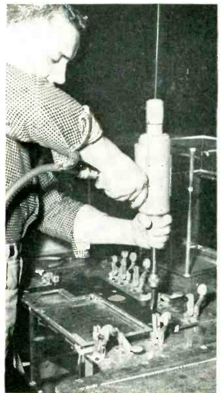
Assembled frame is held by holding fixture built into work bench while riveting panel to frame, using Cherry rivets shown on wire in foreground
