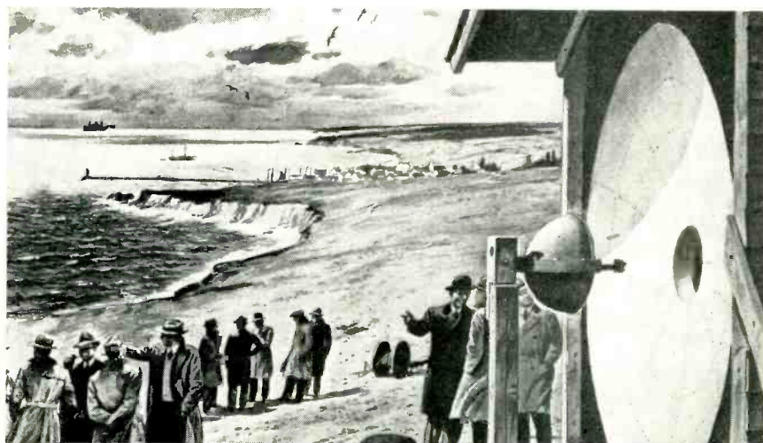
Artist's drawing shows microwave dish antenna used 25 years ago to establish communications between Dover, England and Calais, France. Expected by IT&T scientists to be free of fading, the circuit showed seasonal variations of over-water path. Radio-frequency power was about half a watt at 17 centimeters
