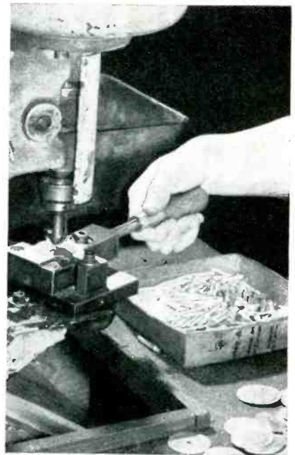
Operator prepares to bring holding fixture into position for reloading after steel shaft has been spun over clutch plate
