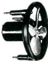
A15AD3 115 Volt 60 cycle axial blower. 35 CFM at .2" static pressure.
