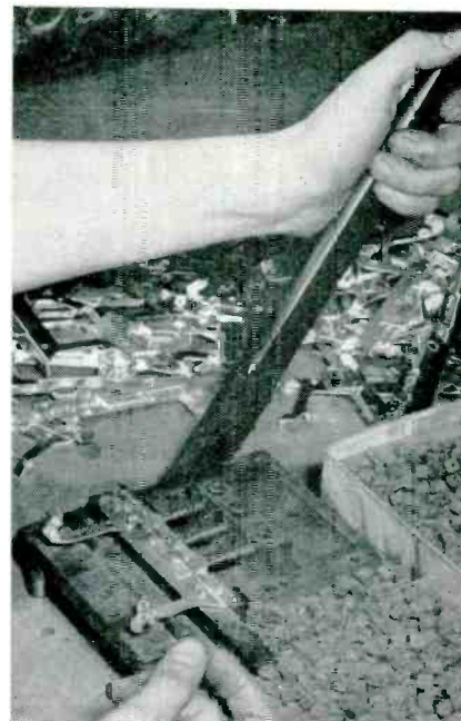
Upper left: Details of grommet-holding fingers. Upper right: Pushing lever back as shown pulls grommets into holes of core bar. Enlarged view below shows that grommets are here just about ready to snap into position in their holes
