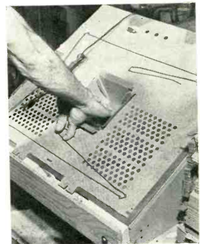
Method of pushing pressed paper cup into hole in back cover
