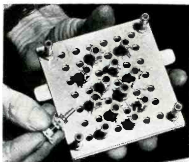
Loading coils into dipping fixture. This fixture holds 42 coils
