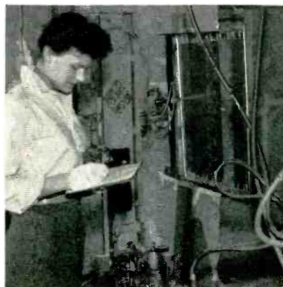
Adhesive spray setup. Photoelectric unit cuts off spray between rack sections
