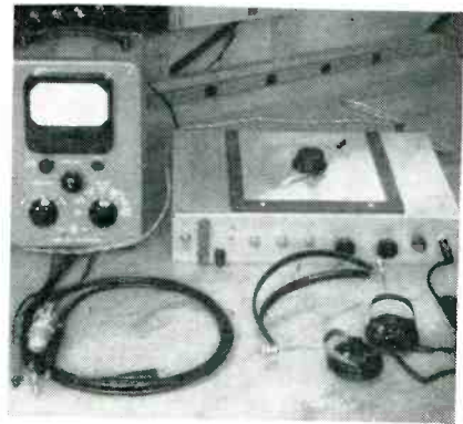
Adapter allows blind to use commercial vtm without circuit modification
