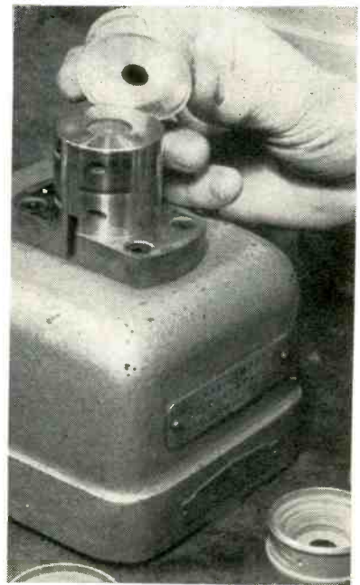
Placing casing on air-leak gage used to check inside diameter of shoulder
