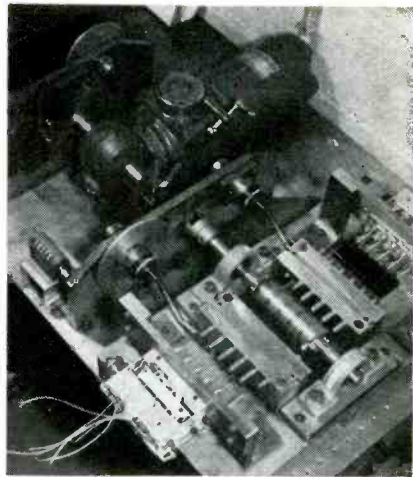
Fixture holding two auto radio pushbutton mechanisms at a time. When set up for use, the central drive shaft of the fixture is hooked up to one end of the universal joint linkages of the drive. Tuners shown here are of the cam-and-lever type
