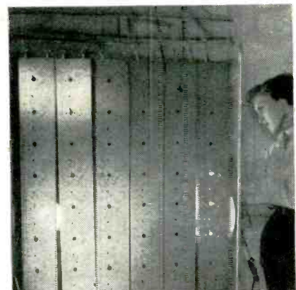
Checking strips for smoothness and coverage of adhesive coating
