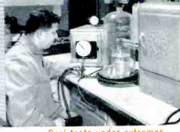
Seal tests under extremes of cold, heat, and altitude.
