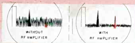
Patterns show signal-to-noise ratio at input to S-band receiver's crystal detector with and without a stage of rf amplification. Utilizing RCA-designed-and-developed type 6861 Traveling-Wave Tube, high signal-to-noise ratio and extended range are obtained. In addition, crystal "burnouts" caused by TR-tube leakage are eliminated by the isolation afforded by the rf stage.
