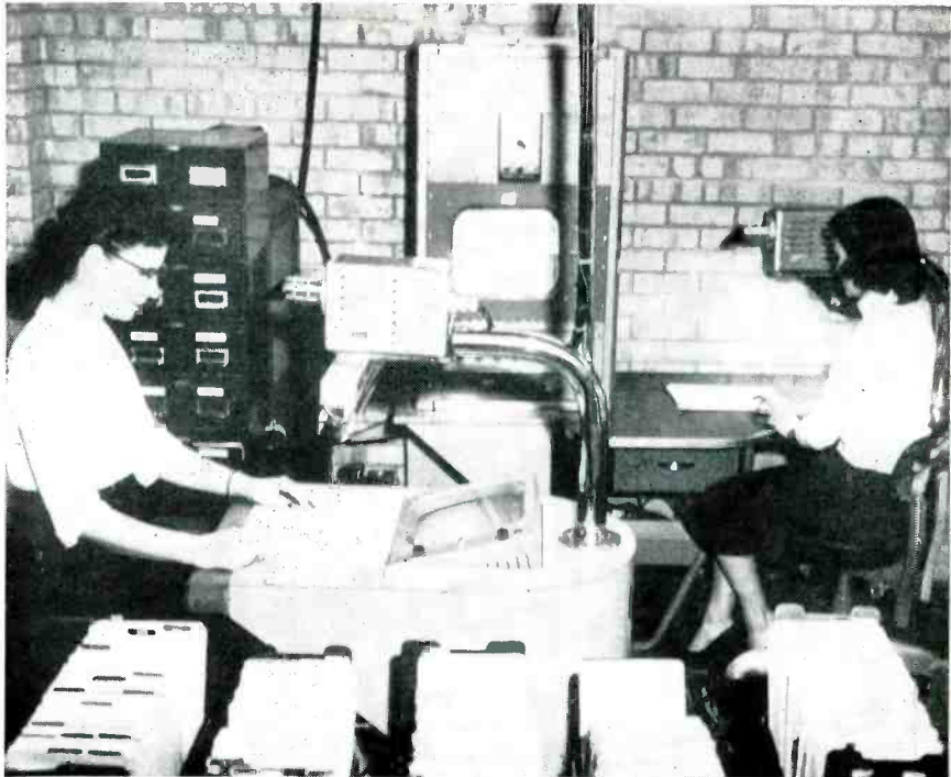
CLERK and Dage industrial tv system ride scooter to view filed bank records. Other new applications indicate . . .
