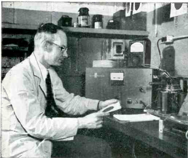
As a Direct-Reading Instrument The extreme sensitivity of the d-c amplifier is utilized to check plasticizer insulation resistance values in the megamegohm range.
