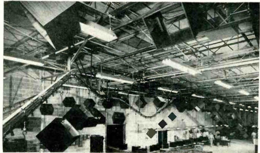
Steel tv cabinets ride overhead conveyors at new Raytheon plant
