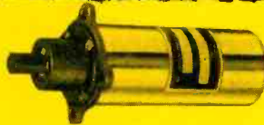
MM or LL motor and planetary gear reducer. Ratios 4-1/3:1 to 21808:1. Torque to 3500 oz.in. Dia. 1 1/4" x 2-7/16" to 4-9/64" long. Bulletin 1000
