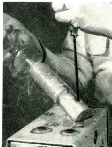
Method of tightening or loosening solder-sealed screw by working through hole in soldering iron
