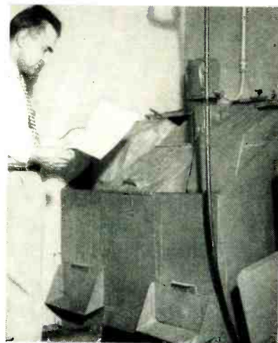
Tumbling machine used in finishing grid cups for electron guns
