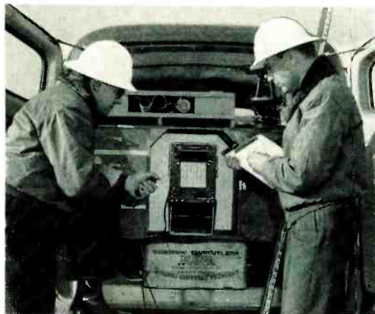
ALI 550-A Oscillographic Recorder being used in the field by Geophysical survey team.
