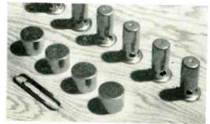
Finished and approved parts after tumbling. Grid cups are below.
