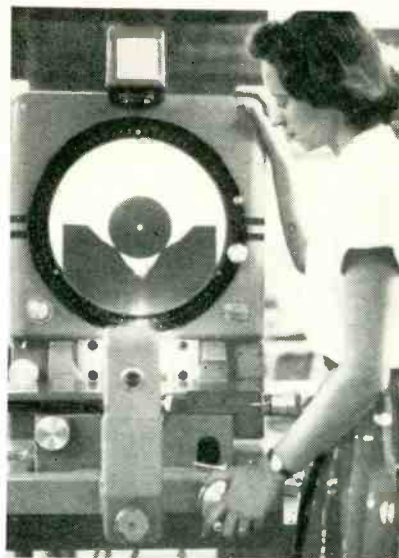
Checking dimensional accuracy of a ten-fold-magnified shadow of a grip cup, using optical magnifier
