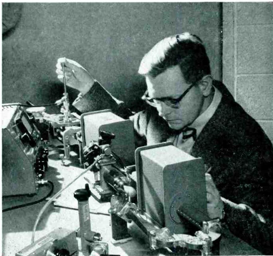
Engineer determining the dielectric constant of a radome wall. A substitution method is used whereby the phase shift produced in an electromagnetic waveform is used to calculate the dielectric constant of the radome material.
