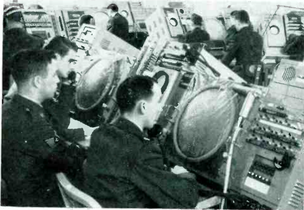
Identification officer and weapons director (left) make decisions on unidentified tracks and guide weapons for interception. Computer maintenance boards (right) check operation of computer circuits
