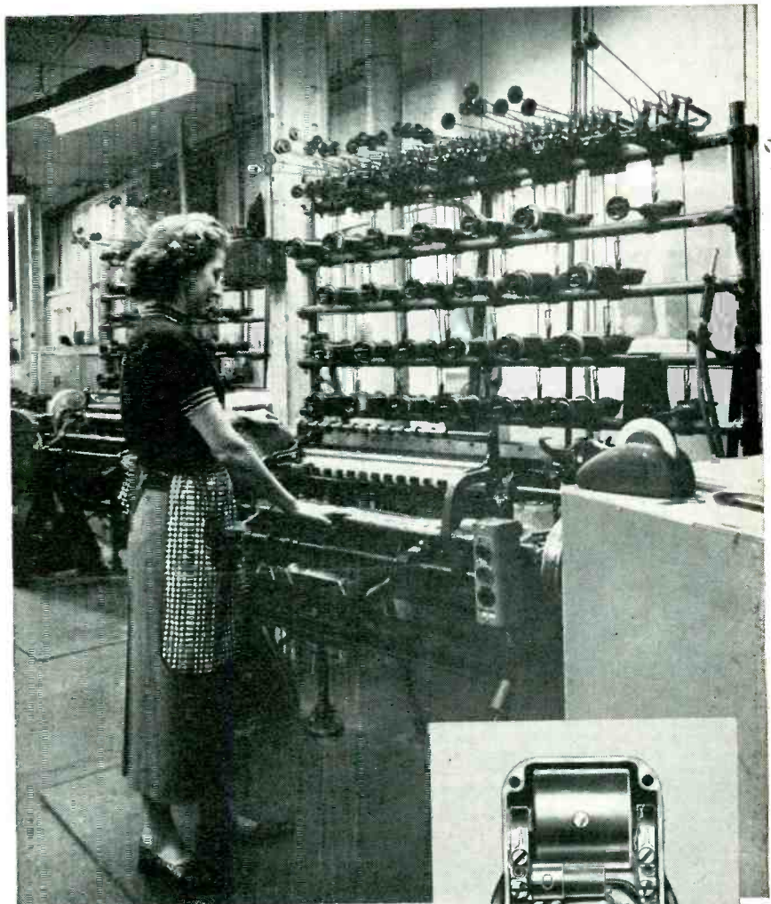
New Leeson No. 107 Automatic Coil Winders, shown in the plant of Wico Electric Company, West Springfield, Mass., were selected because of this firm's long, satisfactory experience with Leeson machines. Leeson No. 107 Winders, featuring speed and accuracy in automatic winding, are creating many plants to boost production and cut costs. Inset shows a cutaway of a Wico Model X Magneto. Coil at top of unit is precision wound on Leeson No. 107's.
