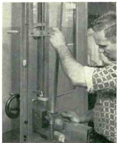
Placing holder containing wound mandrel in fixture used for winding mandrel onto core
