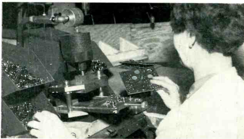
Placing radio board over four sockets loaded into metal slide of press
