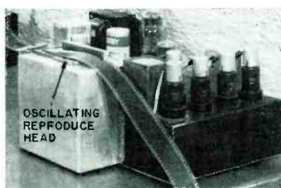
FIG. 7—Auxiliary sync checker with oscillating reproduce head mounted alongside amplifier chassis
